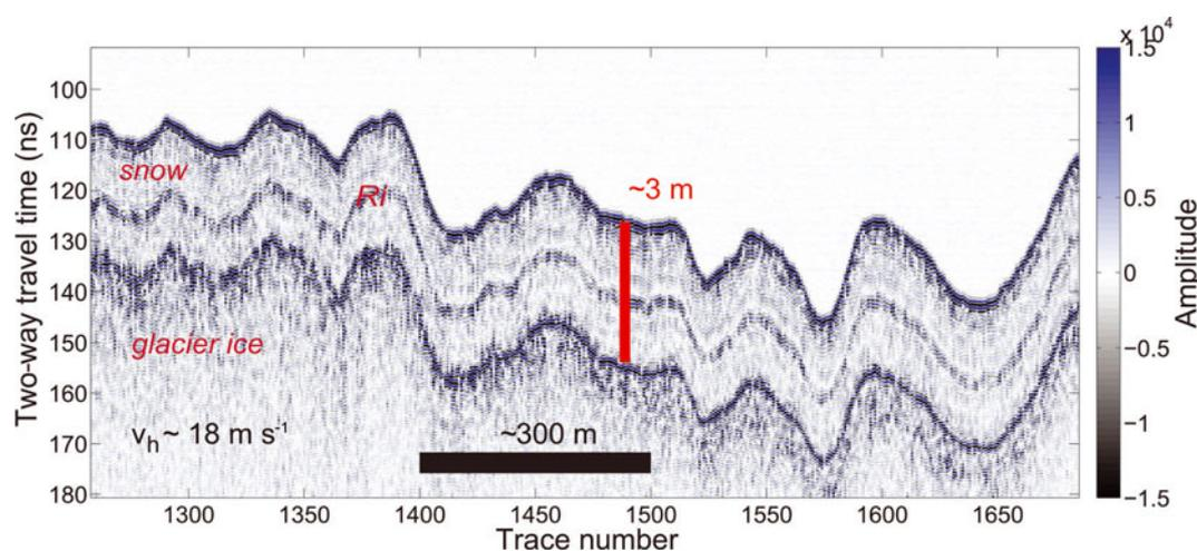
**Fig. 5.** 500 MHz, helicopter-borne GPR image on the ablation area of Scott Glacier, Prince William Sound (location in Fig. 3c). The snowpack imaged is maritime. Data were acquired with a measurement every  $\sim 3$  m. Data clearly display a recognizable internal reflection within the snowpack. Depth scale in the snowpack is for guidance only and was derived using radar velocity of  $0.23 \text{ m ns}^{-1}$ .  $v_h$  indicates helicopter speed.
