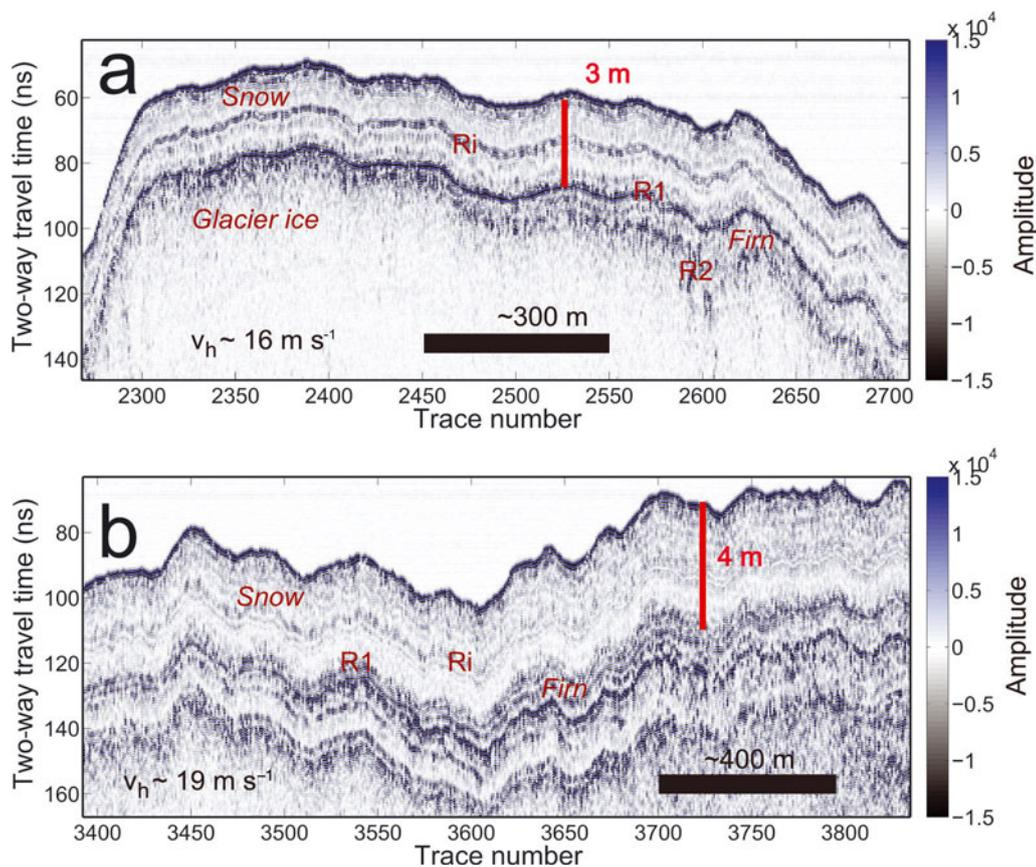
**Fig. 7.** 500 MHz, helicopter-borne GPR image of the accumulation area of Scott Glacier (location in Fig. 3c). (a) The transition from glacier ice to firn, imaged at  $820\text{--}850\text{ m}$  elevation; (b) the sub-horizontal radar stratigraphy in the accumulation area, at  $1020\text{--}1090\text{ m}$  elevation. Depth scales in the snowpack are for guidance only and were derived using radar velocity of  $0.23\text{ m ns}^{-1}$ .  $v_h$  indicates helicopter speed.
