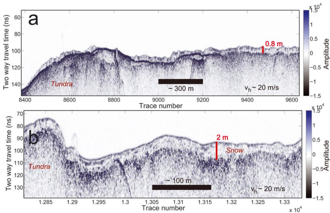
**Fig. 10.** 500 MHz, helicopter-borne GPR image acquired in mountainous tundra terrain in the Alaska Range (location in Fig. 3b).  $v_h$  indicates helicopter speed.
