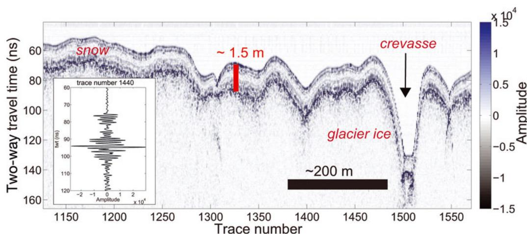
**Fig. 4.** 500 MHz, helicopter-borne GPR image on West Fork Glacier in the Alaska Range (location in Fig. 3a). The snowpack imaged is continental. Data were acquired with a measurement every  $\sim 2$  m. Depth scale in the snowpack is for guidance only and was derived using radar velocity of  $0.23 \text{ m ns}^{-1}$ . Inset shows sample radar trace number 1440. Inset shows sample singular radar trace.
