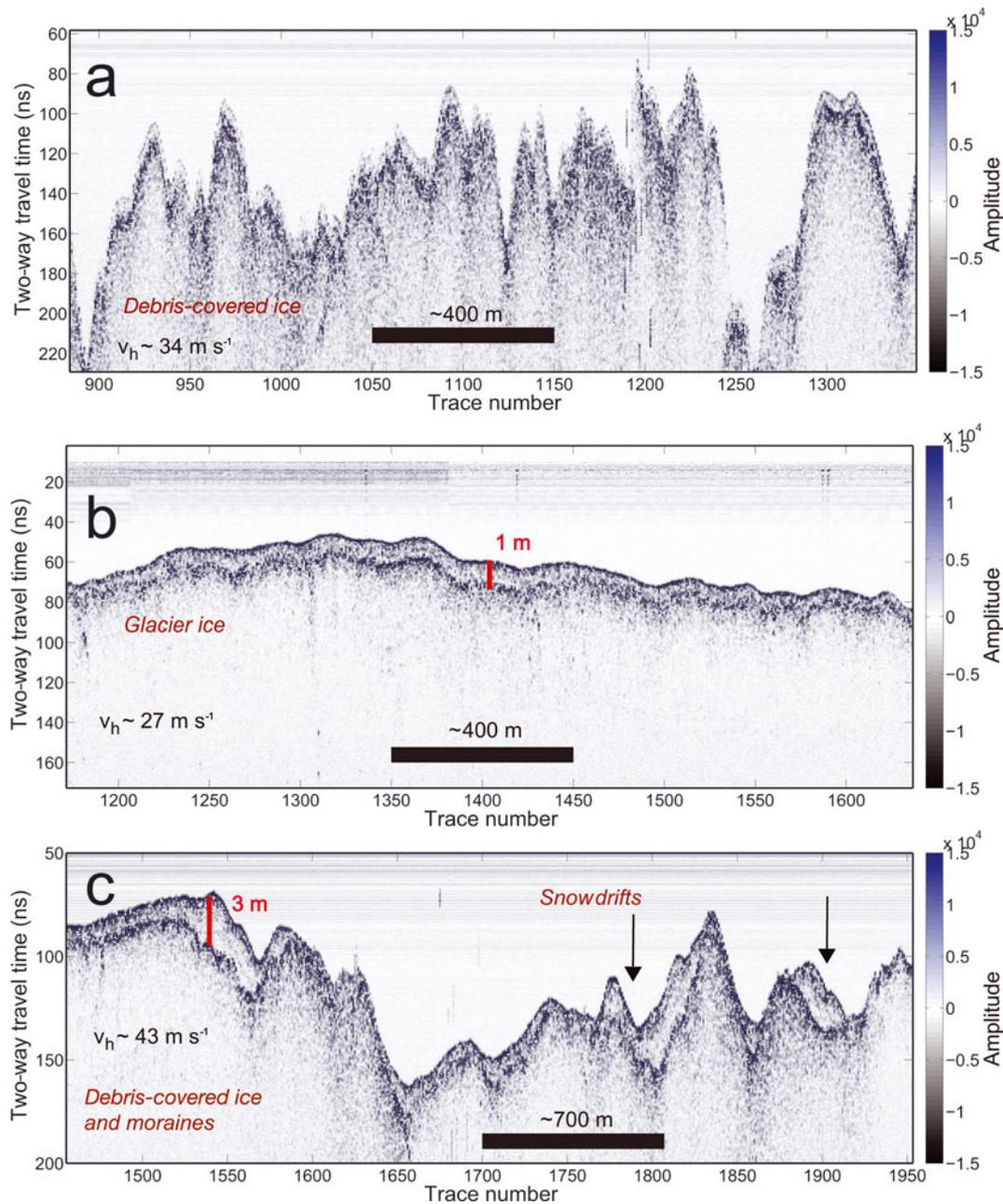
**Fig. 9.** 500 MHz, helicopter-borne GPR images on debris-covered Susitna Glacier in the Alaska Range (location in Fig. 3a). (a) shows the terminus at the lower area (900–950 m), (b) is at 1000–1200 m and (c) is at 1300–1350 m, in an area with large moraines. Depth scales in the snowpack are for guidance only and were derived using radar velocity of  $0.23 \text{ m ns}^{-1}$ .  $v_h$  indicates helicopter speed.
