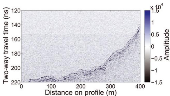
**Fig. 14.** 500 MHz, helicopter-borne GPR image acquired in mountainous tundra terrain in the Alaska Range. The helicopter flying speed was  $\sim 45 \text{ m s}^{-1}$  (more than twice the average speed used in our survey and  $\sim 7$  times faster than previously reported in the literature). At such a high speed, data quality is very low and the reflections from the base of the snowpack are no longer recognizable.
