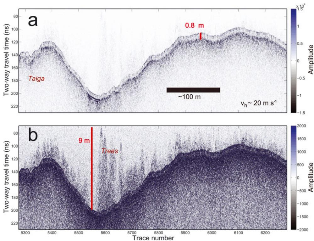
**Fig. 11.** 500 MHz, helicopter-borne GPR image acquired over the boreal forest in the Susitna valley in the Alaska Range (location in Fig. 3b). (a) shows the snow-ground reflector, whereas in (b) the color amplitude scale is modified to highlight returns from the canopy cover. Depth scales in snow and air were derived using radar velocities of  $0.23$  and  $0.3 \text{ m ns}^{-1}$ , respectively.  $v_h$  indicates helicopter speed.
