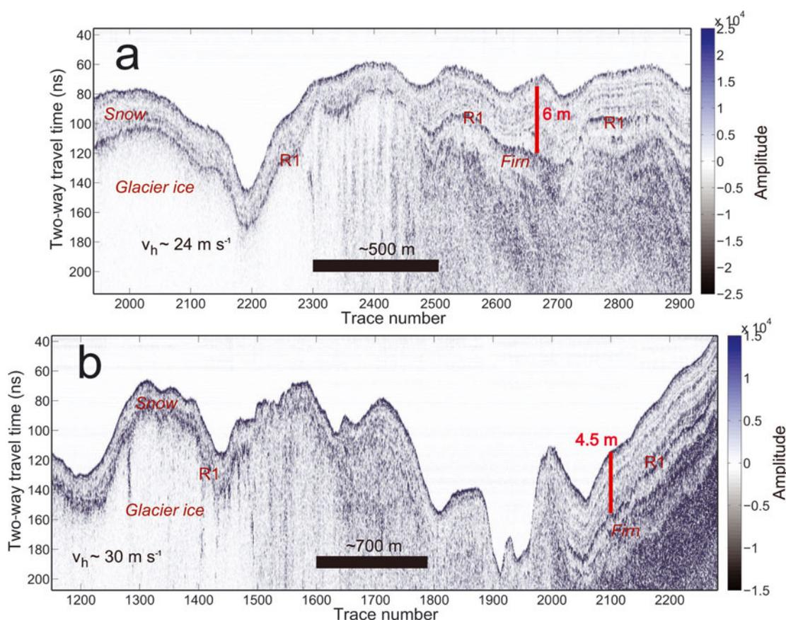
**Fig. 8.** 500 MHz, helicopter-borne GPR images in two different accumulation basins of West Fork Glacier (location in Fig. 3a). (a) was acquired at 1750–2070 m elevations and shows the transition from glacier ice to firn. In (b), acquired at 1850–2100 m elevation, the same transition is not as clear. Depth scales in the snowpack are for guidance only and were derived using radar velocity of  $0.23 \text{ m ns}^{-1}$ .  $v_h$  indicates helicopter speed.
