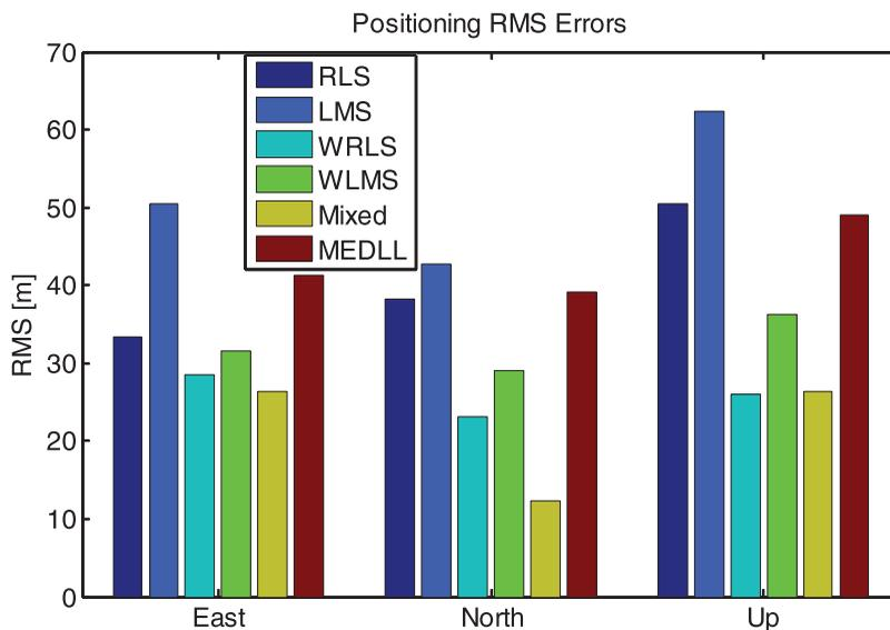
Figure 9. Comparison of position estimation RMS errors.
