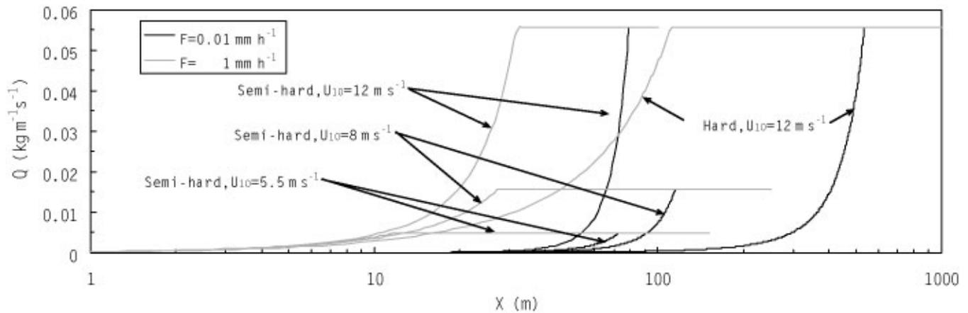
Fig. 5. Change of snowdrift transport rate with fetch distance for drifting snow accompanied by snowfall.
