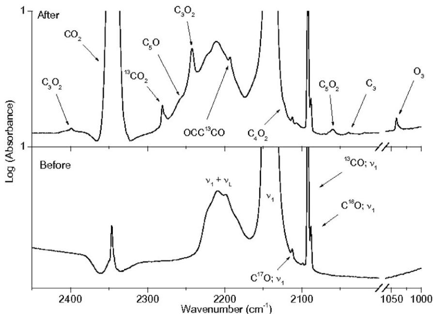
**Figure 1.** Infrared spectrum of CO ice before and after 46 MeV  $^{58}\text{Ni}^{11+}$  irradiation with fluence of  $1.0 \times 10^{12} \text{ cm}^{-2}$ . Many infrared bands were identified by means of their wavenumber positions.
