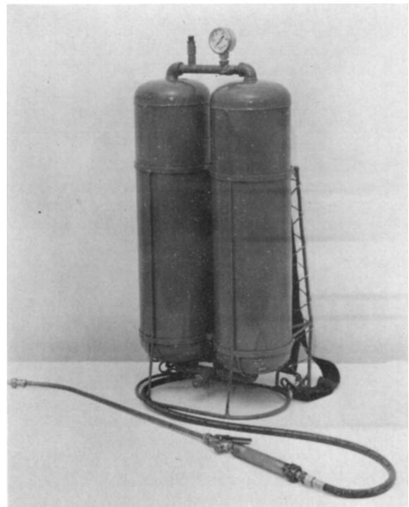
Figure 8. Double-tank pressure knapsack. This double-tank unit is constructed of stainless steel. It incorporates a tank valve, pop-off relief valve and pressure gauge at the top. A quick-coupler injector and pressure regulator are installed at the bottom. The spray is dispersed through the regulator to the hose and gun. Nozzle pressure is 30 psi. Initial air pressure is 30 psi. When liquid is pumped in until the pressure reaches 100 psi, the liquid capacity is five gallons.
