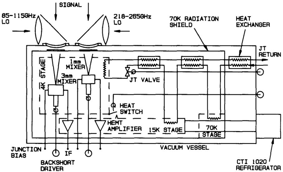
Fig. 1. Cryostat configuration.
