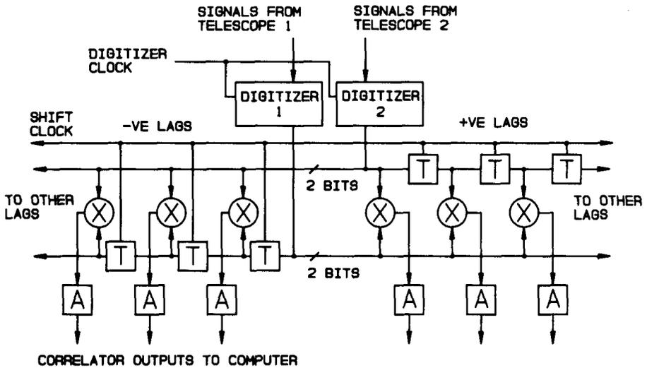
Fig. 2. Digital crosscorrelator architecture. X is a 2-bit multiplier, T is a delay of one shift clock period and A is an accumulator.
