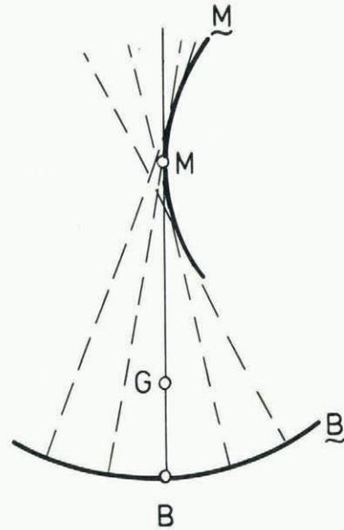
Fig.2.  $B$ , centre of buoyancy;  $\underline{B}$ , buoyancy locus;  $M$ , metacentre;  $\underline{M}$ , metacentric locus;  $G$ , centre of gravity.
