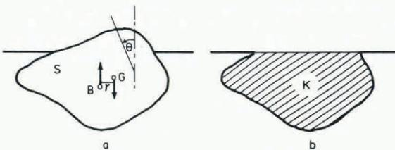
Fig.1. (a) Two-dimensional iceberg of cross-section  $S$  and (b) the fluid it displaces.  $B$ , centre of buoyancy;  $G$ , centre of gravity of  $S$ ;  $r$ , righting arm.
