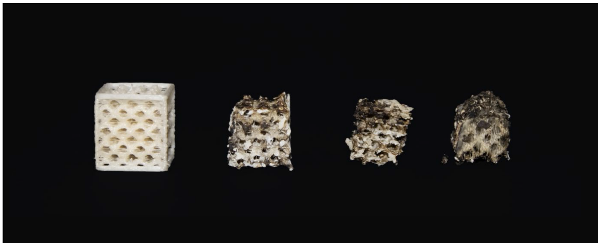
Figure 5. 50% PLA/50% PHBV samples: before composting (left) and after composting at 40°C for 65 days (right, triplicate samples). The composted samples display varying degrees of decomposition, reflecting the heterogeneous nature of microbial colonization
