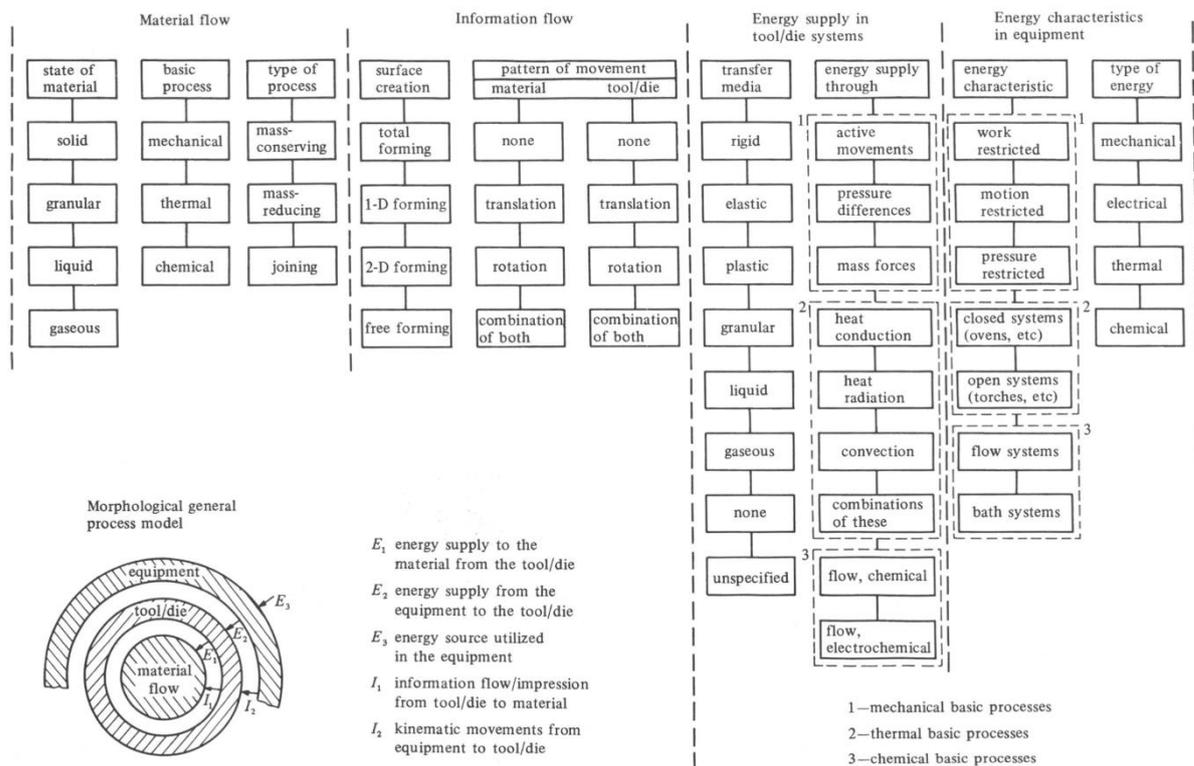
Figure 2. The morphological structure of material processes (Alting, 1978)
