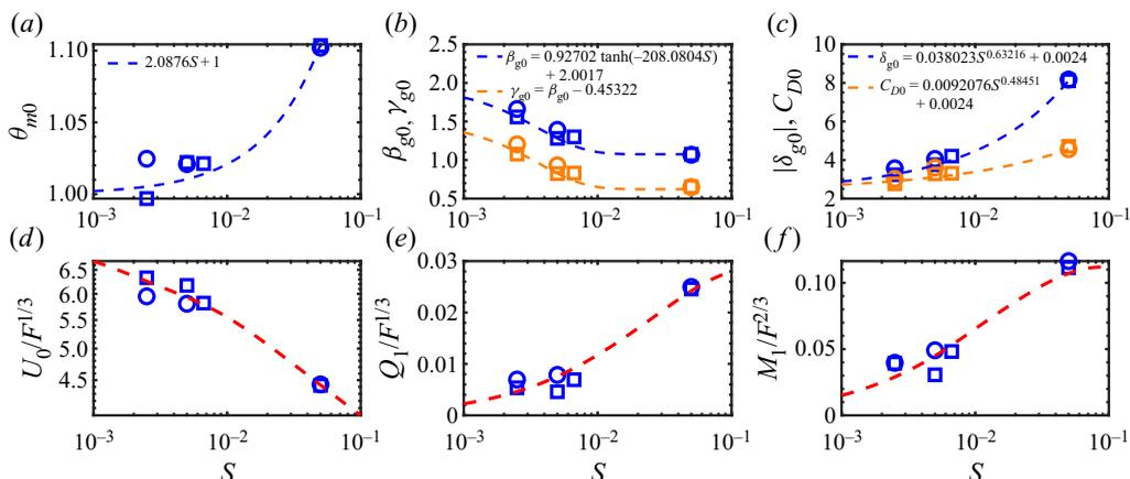
Figure 6. Various near-self-similar shape factors and quantities plotted as a function of bed slope: (a)  $\theta_{m0}$ , (b)  $\beta_{g0}$  and  $\gamma_{g0}$ , (c)  $|\delta_{g0}|$  and  $C_{D0}$ , (d)  $U_0/F^{1/3}$ , (e)  $Q_1/F^{1/3}$  and (f)  $M_1/F^{2/3}$ . The blue dashed and orange dashed lines are best fits of our data; the red dashed lines are derived models (see (2.13a,b) and (2.14)).
