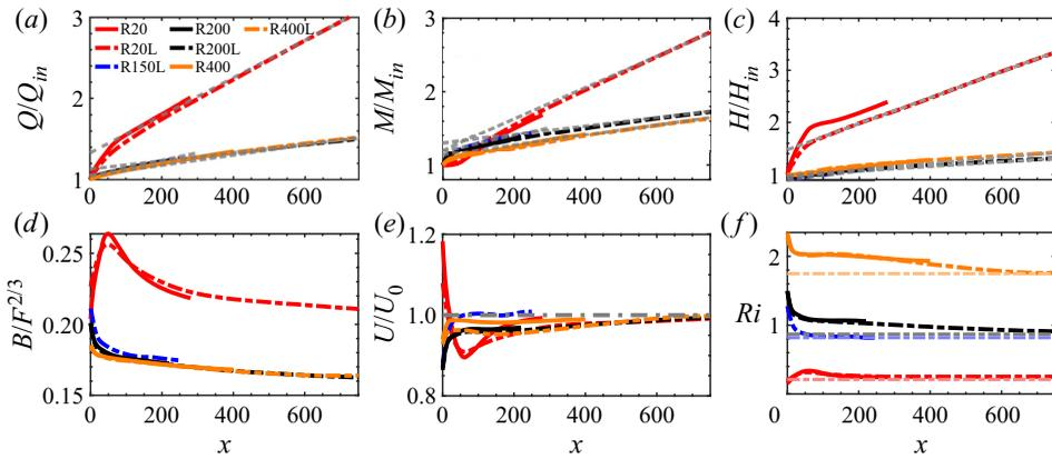
Figure 4. Streamwise evolution of (a)  $Q(x)/Q_{in}$ , (b)  $M(x)/M_{in}$ , (c)  $H(x)/H_{in}$ , (d)  $B(x)/F^{2/3}$ , (e)  $U(x)/U_0$  and (f)  $Ri(x)$ . Dashed grey lines show slopes in the self-similar state obtained from (2.13a,b) and (2.19). Dash-dotted horizontal lines in (f) show  $Ri_0$  for each slope.
