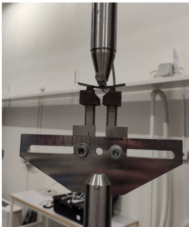
Figure 9. Experimental ASTM D790 standard test setup.
