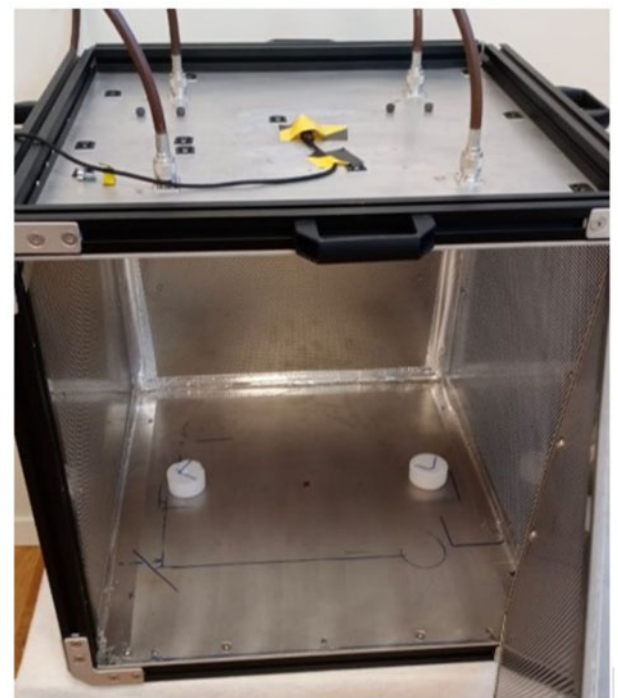
Figure 3. Fabricated multi-mode cavity as applicator.
