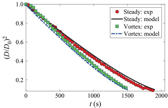
Figure 1. Model validation: comparison of diameter regression,  $(D/D_0)^2$ , between experimental (levitated droplet) and model data. ‘Steady’ represents experiments with no vortical flow. ‘Vortex’ represents experiments with vortical flow over a levitated droplet. In experiments, the initial droplet diameter is  $D_0 = 1.8$  mm.
