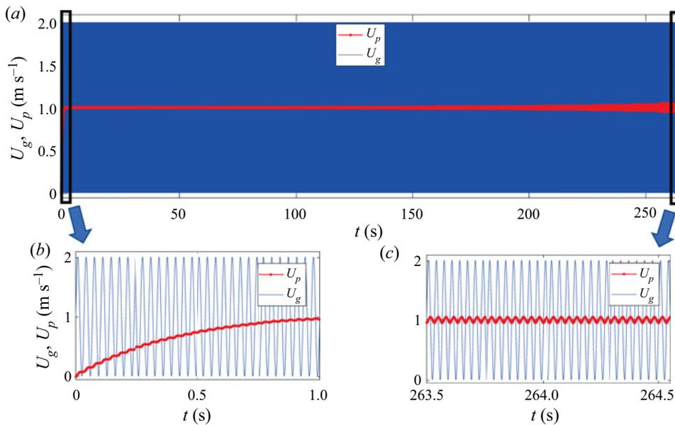
Figure 4. The instantaneous velocities of the gas phase ( $U_g$ ) and the droplet ( $U_p$ ) as functions of time for initial droplet size  $D_0 = 594 \mu\text{m}$ . The gas-phase oscillation has amplitude  $a = 1 \text{ m s}^{-1}$  and frequency of  $f = 30 \text{ Hz}$ .
