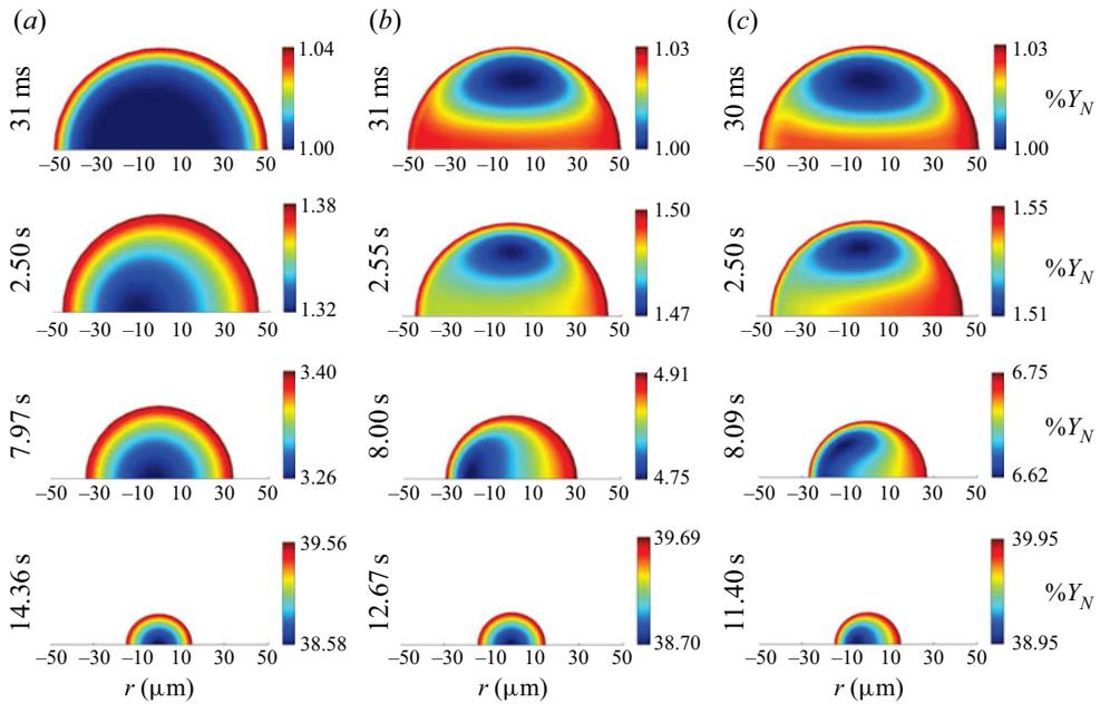
Figure 8. Solute concentration distribution in the liquid phase at different time steps for  $D_0 = 100 \mu\text{m}$  with initial droplet temperature,  $T_0 = 303 \text{ K}$ . The ambient condition is  $T_{\text{amb}} = 301 \text{ K}$  and  $RH_{\text{amb}} = 48 \%$ . The gas-phase perturbation: (a) amplitude,  $a = 0.1 \text{ m s}^{-1}$ , and frequency,  $f = 5 \text{ Hz}$ ; (b)  $a = 1 \text{ m s}^{-1}$  and  $f = 5 \text{ Hz}$ ; and (c)  $a = 1 \text{ m s}^{-1}$  and  $f = 30 \text{ Hz}$ .
