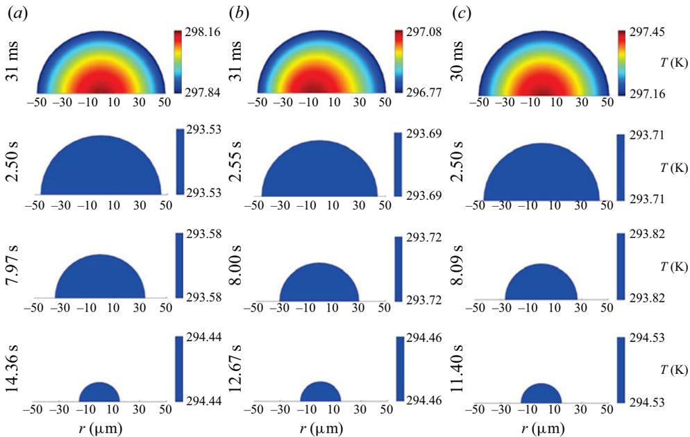
Figure 7. Temperature distribution in the liquid phase at different time steps for  $D_0 = 100 \mu\text{m}$  with initial droplet temperature,  $T_0 = 303 \text{ K}$ . The ambient condition is  $T_{\text{amb}} = 301 \text{ K}$  and  $RH_{\text{amb}} = 48 \%$ . The gas-phase perturbation: (a) amplitude,  $a = 0.1 \text{ m s}^{-1}$ , and frequency,  $f = 5 \text{ Hz}$ ; (b)  $a = 1 \text{ m s}^{-1}$  and  $f = 5 \text{ Hz}$ ; and (c)  $a = 1 \text{ m s}^{-1}$  and  $f = 30 \text{ Hz}$ .
