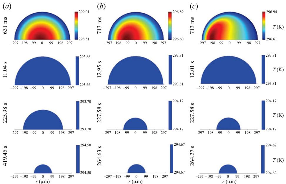
Figure 9. Temperature distribution in the liquid phase at different time steps for  $D_0 = 594 \mu\text{m}$  with initial droplet temperature,  $T_0 = 303 \text{ K}$ . The ambient condition is  $T_{\text{amb}} = 301 \text{ K}$  and  $RH_{\text{amb}} = 48 \%$ . The gas-phase perturbation: (a) amplitude,  $a = 0.1 \text{ m s}^{-1}$ , and frequency,  $f = 5 \text{ Hz}$ ; (b)  $a = 1 \text{ m s}^{-1}$  and  $f = 5 \text{ Hz}$ ; and (c)  $a = 1 \text{ m s}^{-1}$  and  $f = 30 \text{ Hz}$ .
