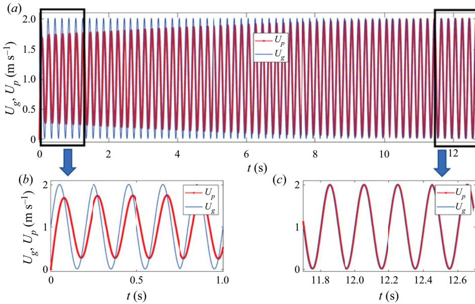
Figure 3. The instantaneous velocities of the gas phase ( $U_g$ ) and the droplet ( $U_p$ ) as functions of time for initial droplet size  $D_0 = 100 \mu\text{m}$ . The gas-phase oscillation has amplitude  $a = 1 \text{ m s}^{-1}$  and frequency of  $f = 5 \text{ Hz}$ .
