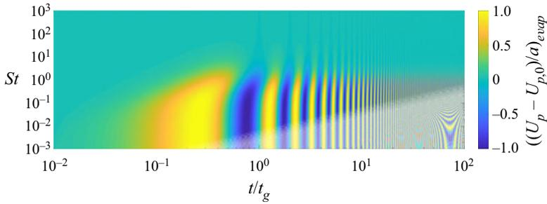
Figure 11. Contour plot of non-dimensional droplet velocity,  $(U_p - U_{p,0})/a$ , with Stokes number ( $St$ ) and non-dimensional time ( $t/t_g$ ), where  $t_g$  is the gas-phase perturbation time. Here, we used the  $d^2$  law to assess the change in evaporating droplet radius.
