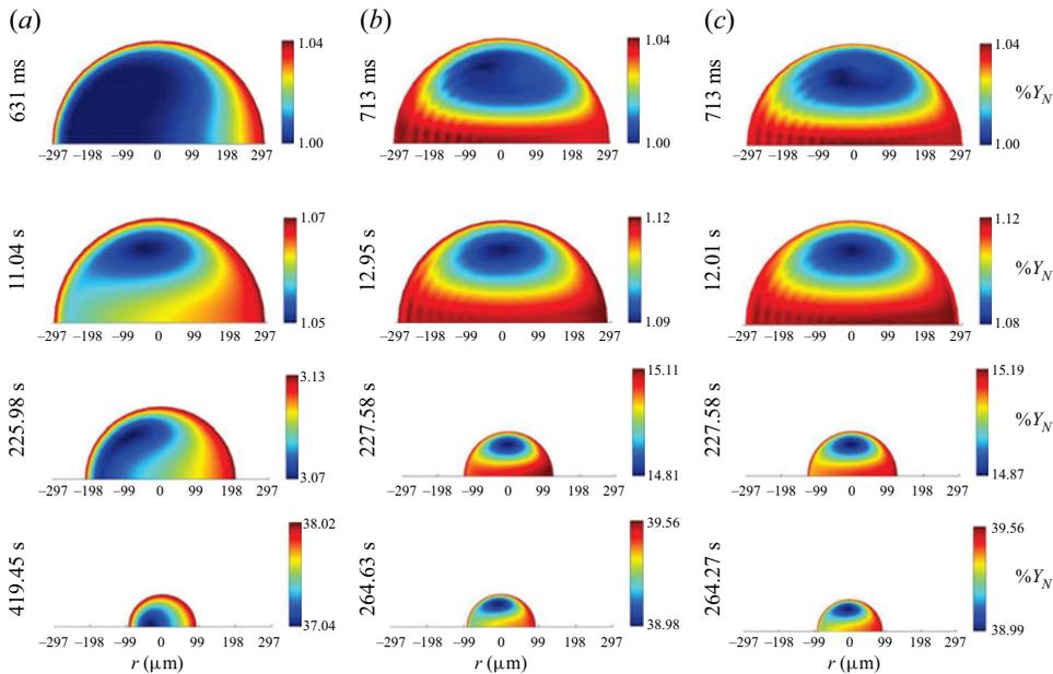
Figure 10. Solute concentration distribution in the liquid phase at different time steps for  $D_0 = 594 \mu\text{m}$  with initial droplet temperature,  $T_0 = 303 \text{ K}$ . The ambient condition is  $T_{\text{amb}} = 301 \text{ K}$  and  $RH_{\text{amb}} = 48 \%$ . The gas-phase perturbation: (a) amplitude,  $a = 0.1 \text{ m s}^{-1}$ , and frequency,  $f = 5 \text{ Hz}$ ; (b)  $a = 1 \text{ m s}^{-1}$  and  $f = 5 \text{ Hz}$ ; and (c)  $a = 1 \text{ m s}^{-1}$  and  $f = 30 \text{ Hz}$ .
