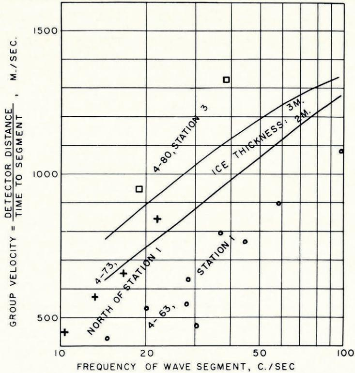
Fig. 5. Dispersion data for flexure waves (theoretical curves from Hunkins (1960, fig. 13))
