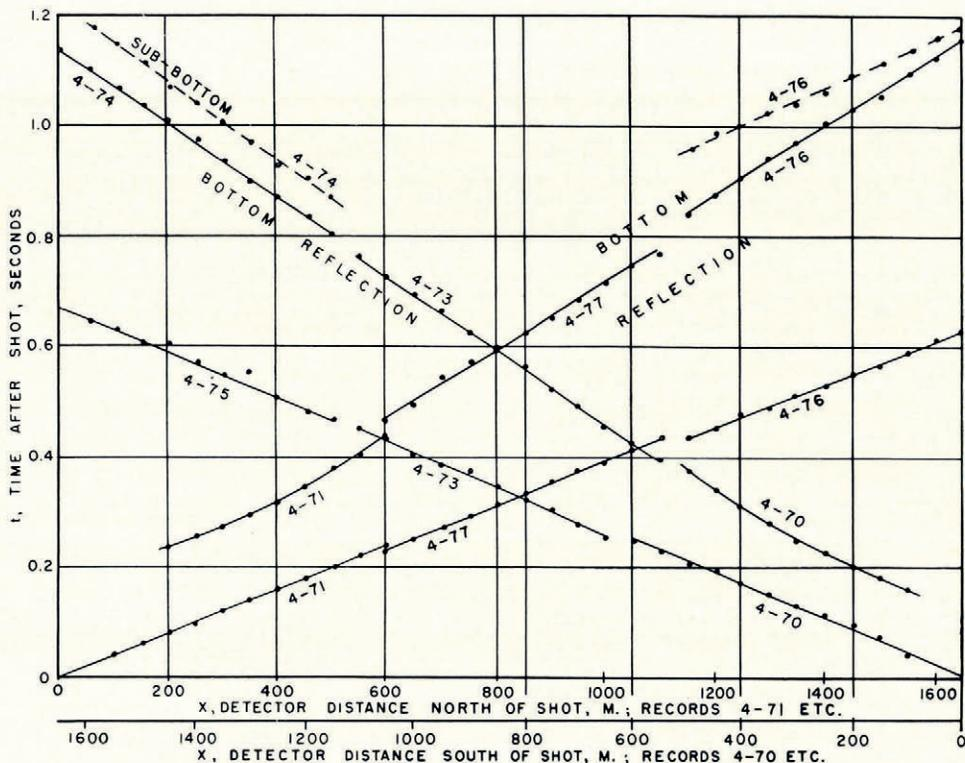
Fig. 3. Travel-time chart for seismograms from station 1
