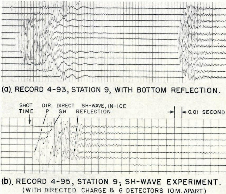
Fig. 6. Typical seismograms from the glacier tongue
