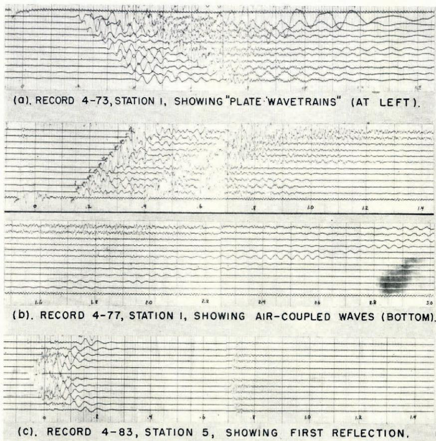
Fig. 4. Specimen seismograms taken on sea ice
