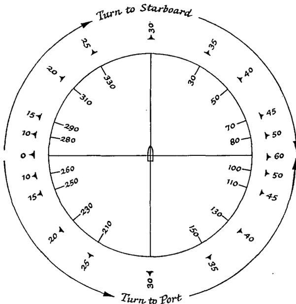
FIG. 1. Hollingdale's rules (rounded). If both ships alter as shown, nearest approach is half the range at which action is taken
