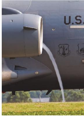
Figure 1. A ground vortex at the engine inlet of a Boeing C-17 Globemaster III during reverse thrust operation visualised by a domain of condensed water vapour within the vortex core (B. Lindsay, 2023, private communication).
