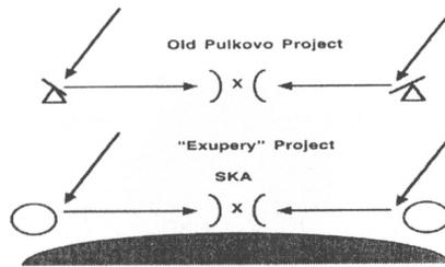
Figure 3. SKA and 'asteroid interferometry'. Collection of the signal from first Fresnel zones, formed on two asteroids by a distant source, with multi-beam SKA instrument. Upper sketch – ground-based analog.
