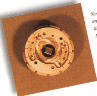
Sample mount: Heater and thermometer are deposited directly on the micro-calorimeter chip for improved sample coupling and reliability.
