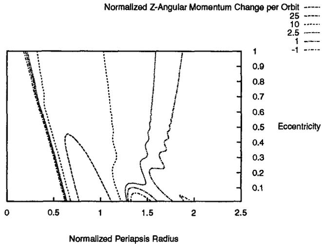
Fig. 2. Normalized  $\Delta H$  per orbit for elliptic orbits (dominant terms only). Multiply contour values by  $-\tilde{C}_{22} \cos^4(i/2) \sin [2(\omega + \Omega)]$  to scale to an arbitrary flyby.
