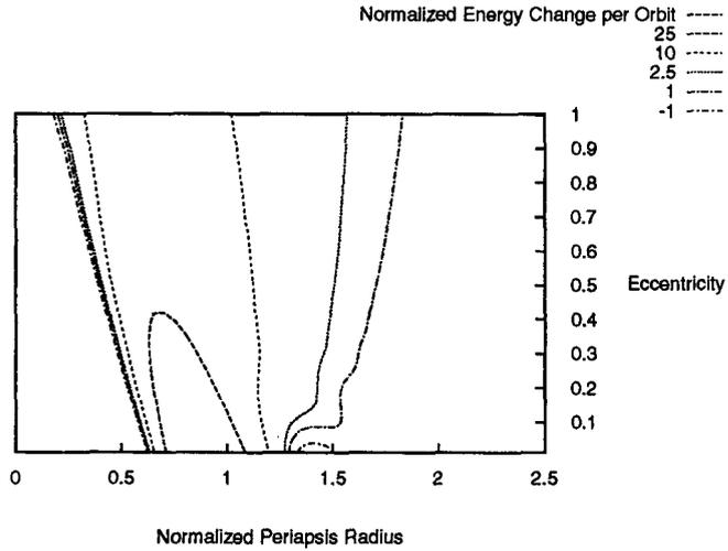
Fig. 1. Normalized  $\Delta C$  per orbit for elliptic orbits (dominant terms only). Multiply contour values by  $-\tilde{C}_{22} \cos^4(i/2) \sin [2(\omega + \Omega)]$  to scale to an arbitrary flyby.
