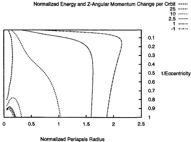
Fig. 3. Normalized  $\Delta C$  and  $\Delta H$  per orbit for hyperbolic orbits (dominant terms only). Note that  $1/e$  is plotted. Multiply contour values by  $-\tilde{C}_{22} \cos^4(i/2) \sin [2(\omega + \Omega)]$  to scale to an arbitrary flyby.
