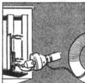
Release of lifebuoy pulls Manoverboard from spring clip, causing it to fall through 90°. As seal breaks internal nylon cords operate two uncocked strikers which ignite smoke candle. Lanyard removes seal from water-activated batteries which have remained watertight during stowage.
