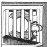
The Manoverboard, connected to lifebuoy, is mounted in the inverted position for protection against sun, weather, etc. Aluminium and polythene construction is corrosion-free.
