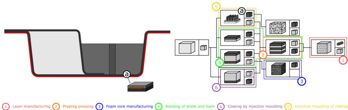
**Figure 5. Hybrid profile with integration of conductor as an insert (left) and resulting multi-level structure including the manufacturing processes (right)**
