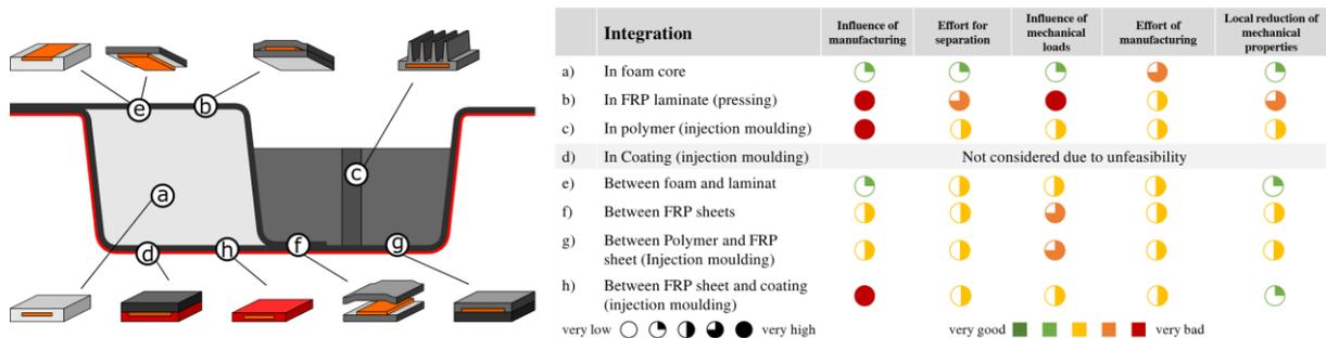
Figure 7. Possible positions of conductive inserts with different influences by manufacturing
