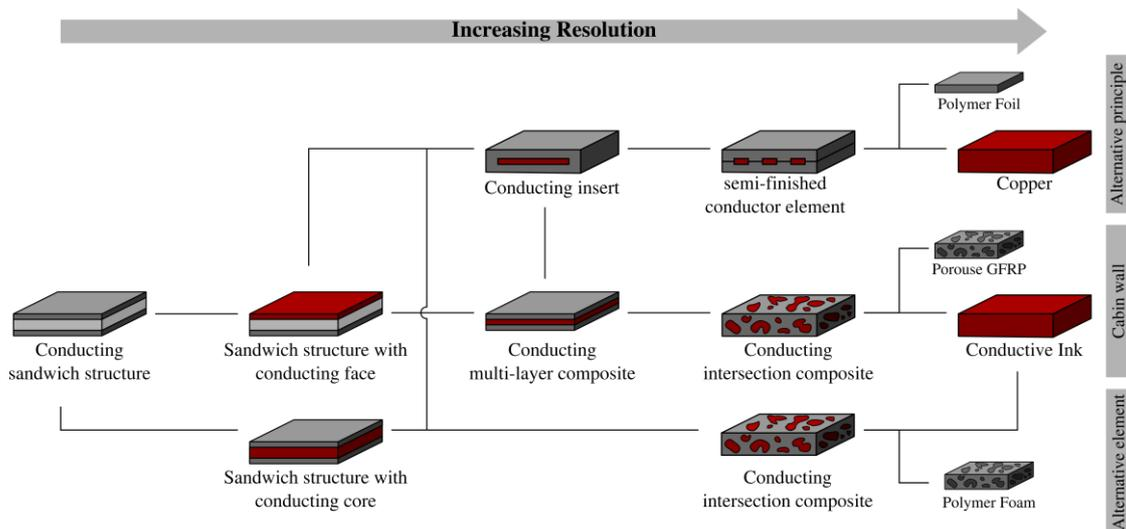
**Figure 4. Principle of linking solutions with different resolutions**
