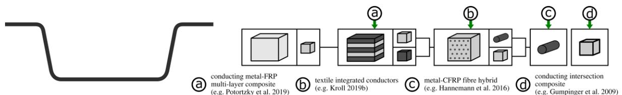
**Figure 6. Multi-functional solutions basing on specific design principles**
