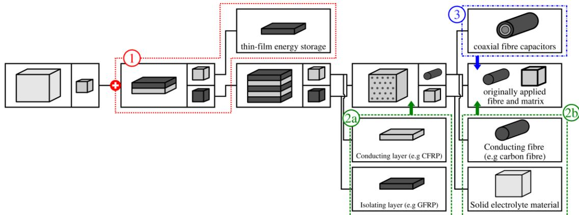
**Figure 3. Example of a multi-level structure at the example of a integration of a structural battery into FRP on different level applied to the example of Adam et al. (2018)**
