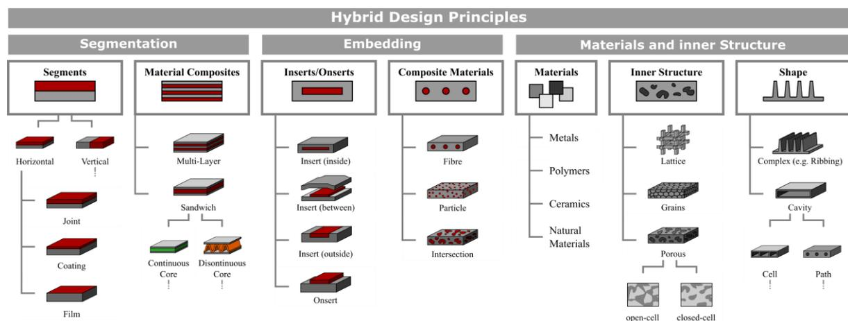
Figure 1. Categorization of design principles for hybrid design and functional integration
