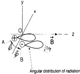
Fig. 2 Radiation emission from an electron and positron moving along field line OB.
