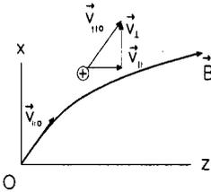
Fig. 1 Particle motion along field line OB.
