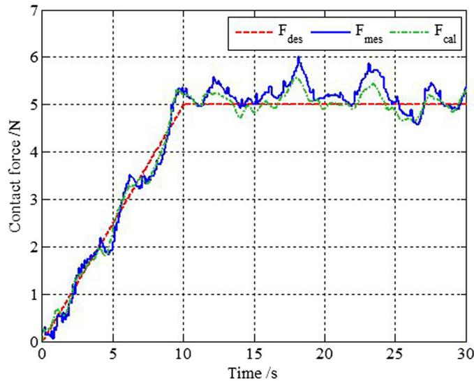
Fig. 15. Ramp force tracking and constant force control.
