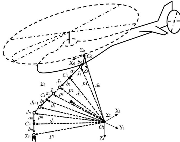
Fig. 9. Frames of AM system based on the centralized approach.
