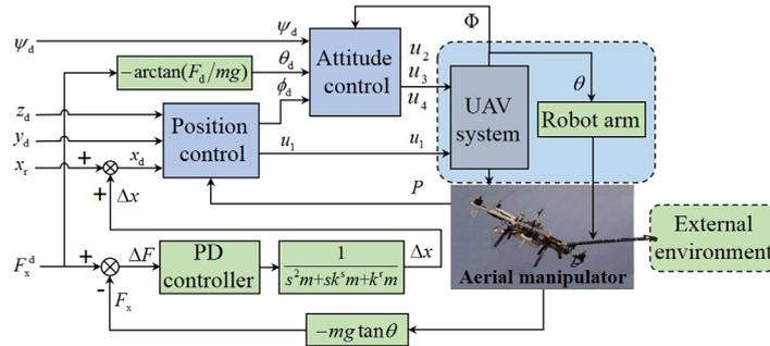
Fig. 13. Contact force control block diagram of AM.
