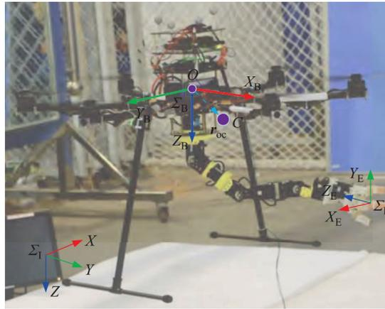
Fig. 7. Frames of AM system based on the separated approach.
