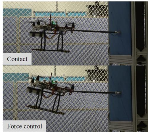
Fig. 14. The contact force control experiment with a quadrotor AM.
