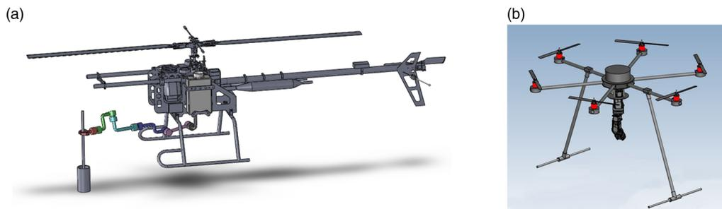
Fig. 2. Aerial manipulation examples. (a) Unmanned helicopter aerial manipulator (Yale University,<sup>8</sup> DLR,<sup>9</sup>) (b) Multirotor aerial manipulator (University of Pennsylvania,<sup>10</sup> Drexel University,<sup>11</sup>).
