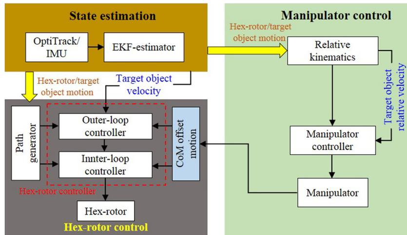
Fig. 8. Control structure of AM system based on decentralized approach.
