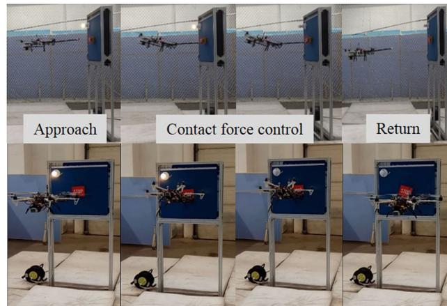
Fig. 17. The process of pressing an emergency switch.
