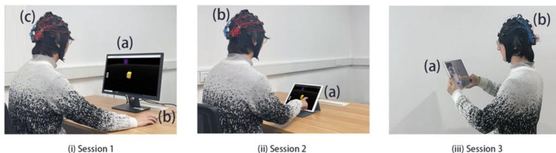
Fig. 2. The experimental settings based on (i) Session 1: mouse-based desktop, (ii) Session 2: touch-based tablet, and (iii) Session 3: handheld AR.
