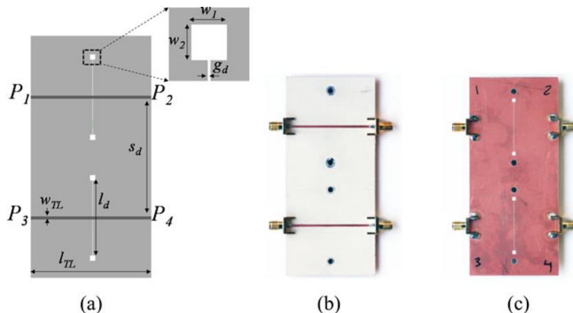
**Fig. 1.** The proposed DB-DGS-based differential sensor. (a) Layout of the microwave part; (b) fabricated device (top); (c) fabricated device (bottom). Dimensions (in mm) are:  $w_1 = w_2 = 2$ ,  $w_{TL} = 1.14$ ,  $l_{TL} = 50$ ,  $l_D = 28$ ,  $g_d = 0.2$ , and  $S_d = 44$ . The considered substrate is the Rogers RO3010 with thickness  $h = 1.27$  mm, dielectric constant  $\epsilon_r = 10.2$ , and loss tangent  $\tan\delta = 0.0035$ .
