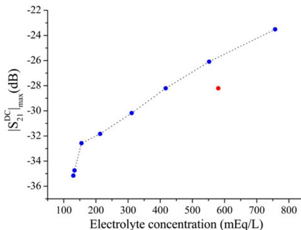
**Fig. 6.** Maximum value of the cross-mode transmission coefficient for the different samples, as inferred from the sensor reported in [39].
