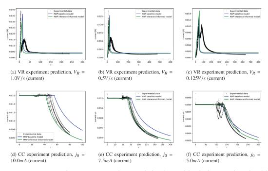
**Figure 14.** Comparisons between current prediction on the baseline model and inference-informed model at the MAP for each.
