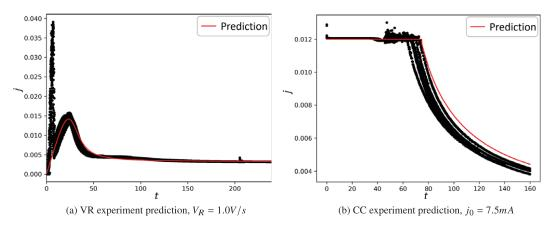
Figure 12. Current prediction on the machine-learning augmented model trained without the first peak model, shown for (a) VR experiment with  $V_R = 1.0 \text{V/s}$  and (b) CC experiment with  $j_0 = 7.5 \text{ mA}$ .
