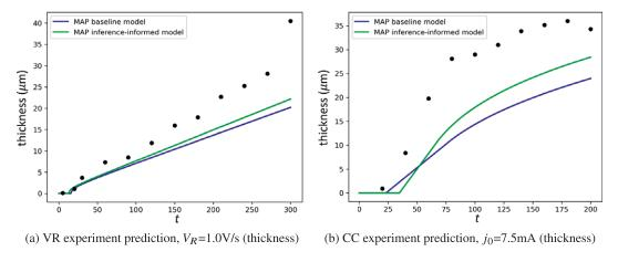
**Figure 9.** Comparisons between film thickness prediction on the baseline model and inference-informed model at the MAP for each.
