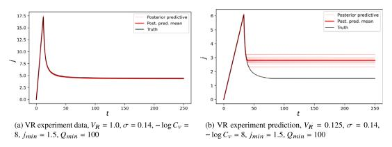
**Figure 6.** Posterior predictive results after performing Gaussian VI on data from a simulated VR experiment. The posterior predictive results in accurate simulations on the data (a), but poor predictions for other experiments (b). This is caused by unidentifiable  $j_{min}$  in the data.
