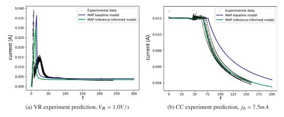
**Figure 8.** Comparisons between current prediction on the baseline model and inference-informed model at the MAP for each on (a) VR experiment with  $V_R = 1.0V/s$  and (b) CC experiment with  $j_0 = 7.5$  mA.
