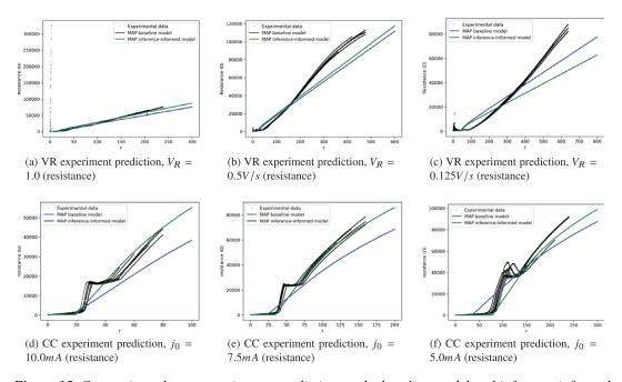
**Figure 15.** Comparisons between resistance prediction on the baseline model and inference-informed model at the MAP for each.
