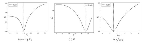
Figure 7. Negative log-likelihoods computed from simulated data on a VR experiment using the inference-informed model with experimental conditions  $V_R = 0.125$ ,  $\sigma = 0.14$ ,  $-\log C_v = 8.5$ ,  $Q_{\min} = 100.0$  (K = 23.2), and  $j_{\min} = 1.5$ .
