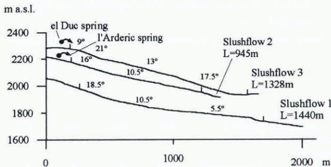
Fig. 3. Topographic profiles of the slushflow paths. *L* is the length of the flows. Starting locations and runouts are shown by vertical lines. Starting zones of slushflows 2 and 3 were associated with sporadic springs. Slope angles represent the different sections of the paths, and do not correspond to the mean inclinations of the starting zones, tracks and runout zones.
