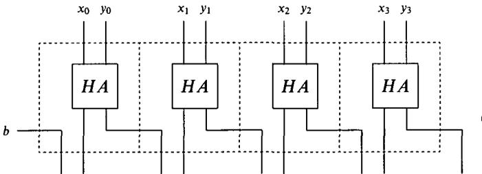
The component  $HA(x, y) = ((x + y) \bmod 2, (x + y) \text{div } 2)$  above is usually called a *half-adder*. If a large number of binary additions are to be done (such as in a multiplier circuit), a considerable speed-up can be obtained by first converting to carry-save numbers, and then doing all the additions using carry-save adders. Using this technique, the carry propagation which occurs when the final carry-save number is converted back to binary is amortized over many additions.
