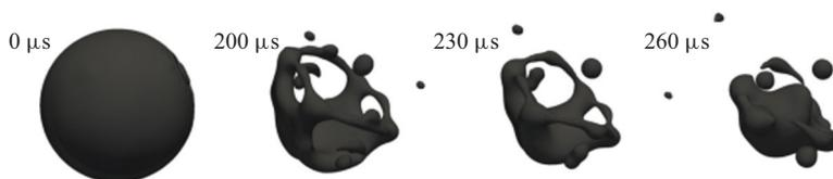
Figure 21. Microexplosion of HFO droplet at  $\alpha_r = 0.7$ .
