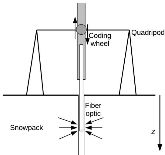
Fig. 3. Schematic illustration of the irradiance profiler SOLEXS.
