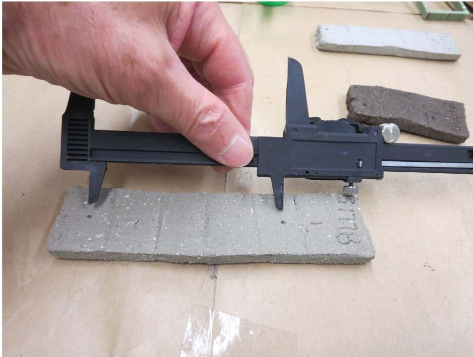
**FIGURE 5.** Marking bar with 10-cm distance with metric calipers for percent Linear Drying Shrinkage measurement.
