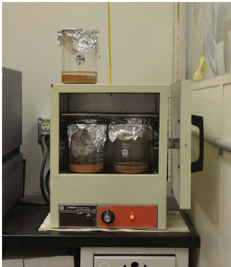
FIGURE 12. Beakers of fine fractions in drying oven (another sample, waiting for space in the oven, is sitting on top, getting a head start on the drying process).
