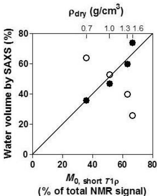
FIG. 4. Relative volumes of IL and non-IL water (in % of total water content) determined by SAXS vs. the magnetization  $M_0$  vector associated with short  $T_{1\rho}$  relaxation times determined by NMR. Filled and open circles refer to the relative volumes of IL and non-IL water, as determined by SAXS.
