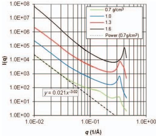
FIG. 5. The intensity as a function of the scattering vector  $q$  for MX-80 samples of different density (in the legend). The intensities have been vertically shifted in order to separate them in the figure. A fitting curve to  $I(q)$  at low  $q$  values is shown for the density  $0.7 \text{ g/cm}^3$ .
