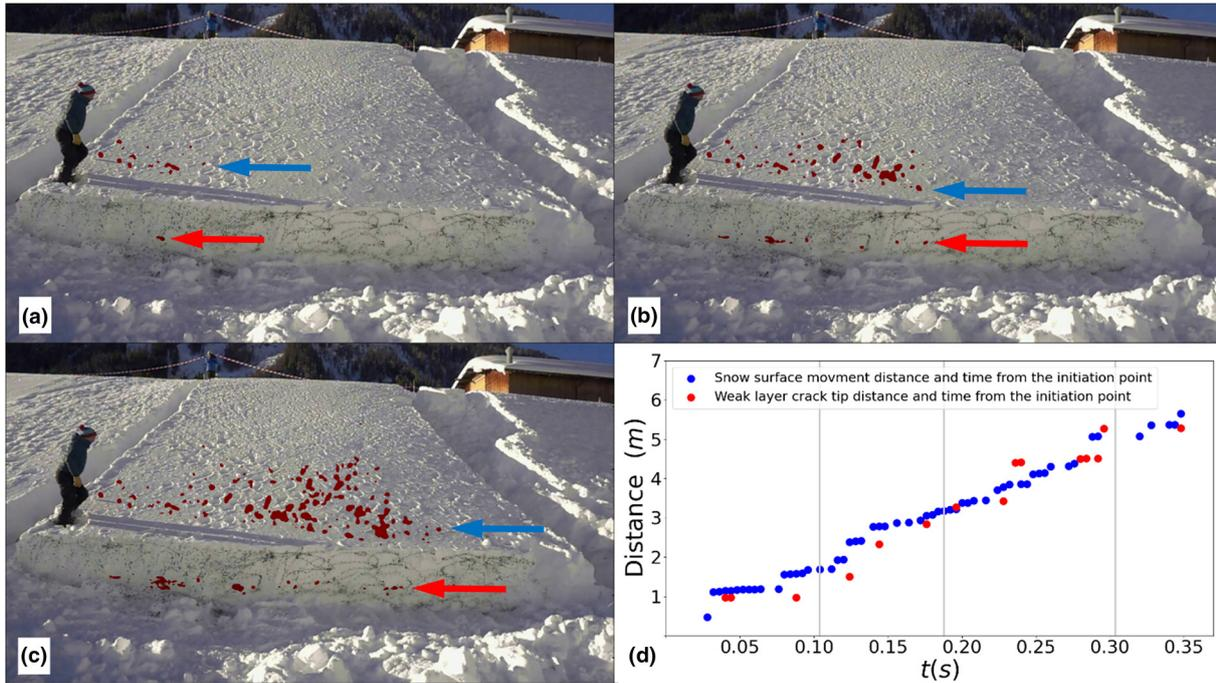
**Figure 2.** A sequence of of a 10 m by 10 m small avalanche experiment video frames where both snow surface movements (marked in blue arrow) and weak layer cracks have been detected (marked in red arrow) after 0.1 s (a), 0.18 s (b) and 0.3 s (c). (d) distance and time from the initiation point and time for both detected snow surface motion (blue) and detected weak layer crack tip (red). The gray vertical lines in D show the time of frames A, B and C.
