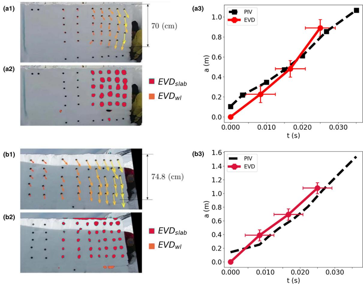
**Figure 5.** (a) Application of the EVM method to field experiments and comparison with results obtained with particle tracking velocimetry (PTV). (a1) PTV results for a flat (0° slope) field PST. (a2) corresponding EVD. (a3) Crack tip position with time-based from PTV (black) and EVD (red). (b) same as (a) for a PST on a 37° slope.
