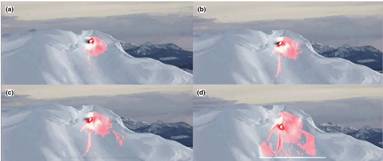
**Figure 8.** A sequence of video frames of avalanche release. In red are the locations where we detected snow surface movement up to the time of the frame. Initially (A and B), weak layer crack propagation can only be detected advancing downslope from the snowboarder. As larger areas of the weak layer fractured downslope from the snowboarder, crack propagation advances in the cross-slope direction.
