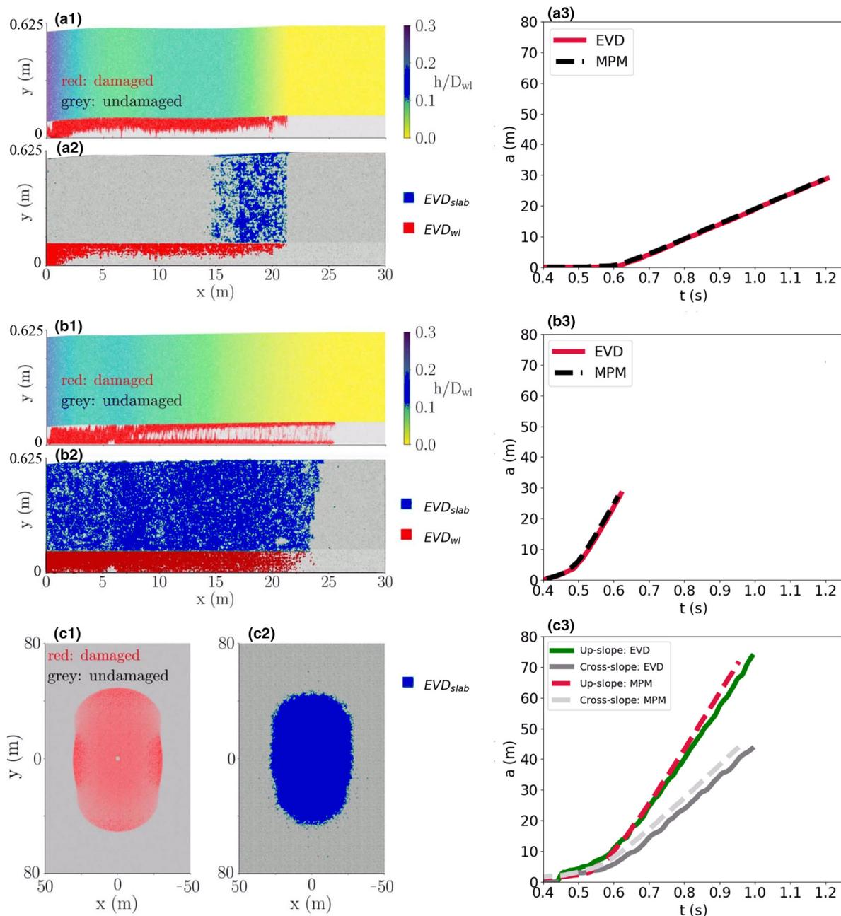
**Figure 7.** (a1) MPM simulation of a 30 m PST on flat terrain, (a2) EVD results for the simulation, and (a3) crack tip position with time-based on MPM (red) and EVD (blue). (b) Same as a) except on a 30° slope. (c1) MPM 2D MPM simulation of an avalanche on 30 degrees slope, (c2) EVD results for the simulation, and (c3) crack tip position with time-based from MPM and EVD in both slope and cross-slope directions.
