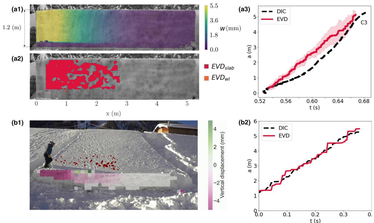
**Figure 6.** (a) Digital Image Correlation (DIC). (a1) PTV results for a flat (0° slope) field PST. (a2) corresponding EVD. (a3) Crack tip position with time-based from DIC (black) and EVD (red). (b1) EVD results on the snow surface (red) on an experiment on a small isolated slope. DIC results for the sidewall facing the camera (colors). (b2) Crack tip position with time from DIC (black) and EVD (red).
