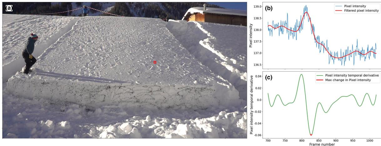
**Figure 4.** (a) A video frame of a 10 m by 10 m small avalanche experiment. (b) The mean pixel intensity (in blue) and the filtered signal (in red) of the pixels in the red rectangle. (c) The first temporal derivative of the filtered pixel intensity signal. The derivative minima (red dot) at frame 828 represented when the weak layer's crack passed below the area marked with the red rectangle. Both (b) and (c) share the same x-axis.
