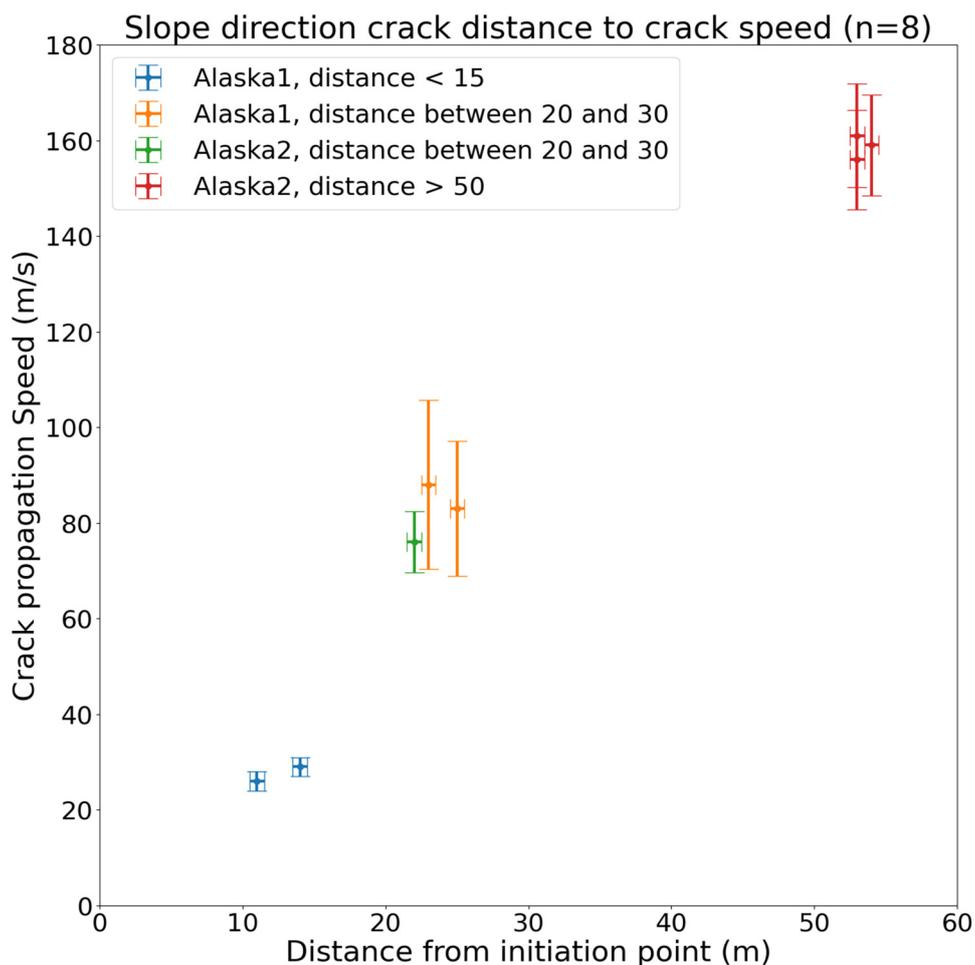
**Figure 10.** Crack propagation speed against crack propagation distance from two videos of a snowboarder-triggered soft slab avalanche (Table 2, Alaska1 and Alaska2), where we could estimate the propagation speed in several distances in one avalanche. The different colors are for the two different avalanches and for different distances from the trigger point of the slide.
