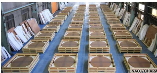
**Figure 4.** Crearceram glass ceramics blanks are in full production for TMT's primary mirror in Japan. These 1.52-m circular discs go through stages of grinding, aspherical polishing, hexing, mounting before going overseas for final touch up, and eventually to the telescope site. TMT needs 594 of such segments. This is another example of utilizing what is available in the industry to specialize to match the research needs.
