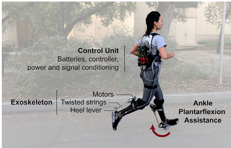
Figure 1. Overview of system components. The user wears an ankle exoskeleton around the shank and foot that applies ankle plantarflexion assistance torques. A control unit is carried on the user's back.
