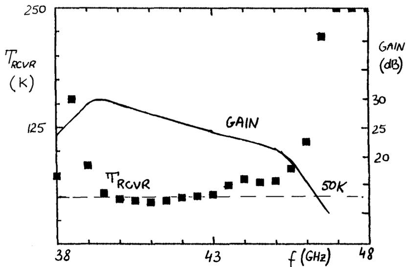
Fig. 3. Noise performance of the laboratory version of the Q-band receiver. Gain of the cryogenic amplifier is also plotted.
