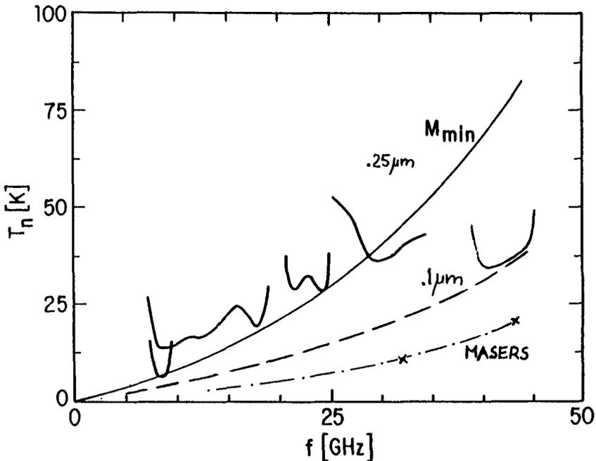
Fig. 1. Noise temperature of different amplifiers and minimum noise measure of FHR02X ( $.25\ \mu\text{m}$  gate length) and H-CF-100-6 ( $.1\ \mu\text{m}$  gate length) at  $T_n = 12.5\ \text{K}$ . The noise performance of masers at 4 K is also shown for comparison.
