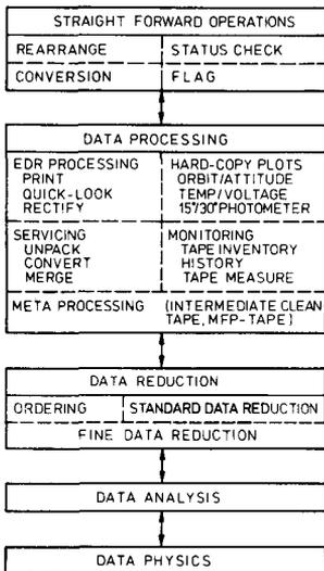
Figure 2 - Experimenter Data System-Processing Levels
