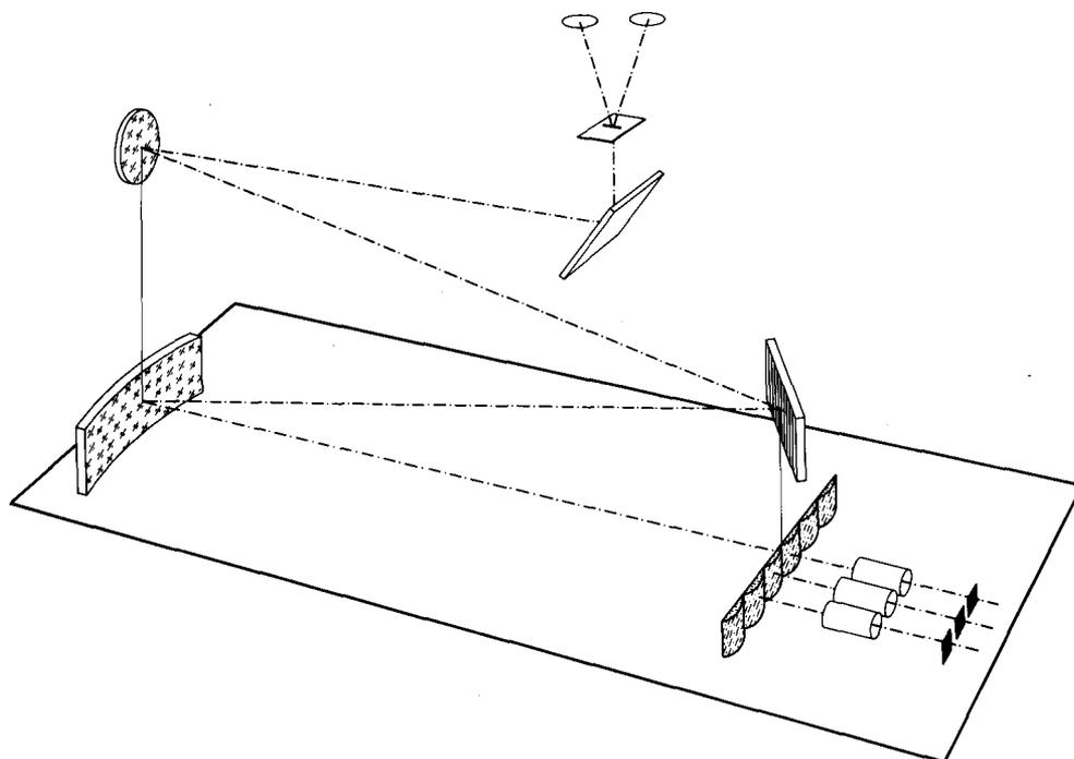
Fig. 10 Principle of a "multi" white pupil spectrometer using the field slicing technique
