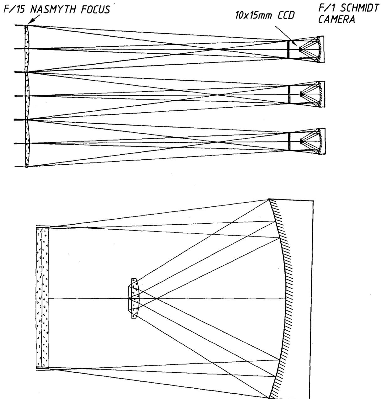
LARGE FIELD IMAGING AT NASMYTH FOCUS USING THE FIELD SLICING TECHNIQUE (F/1)
