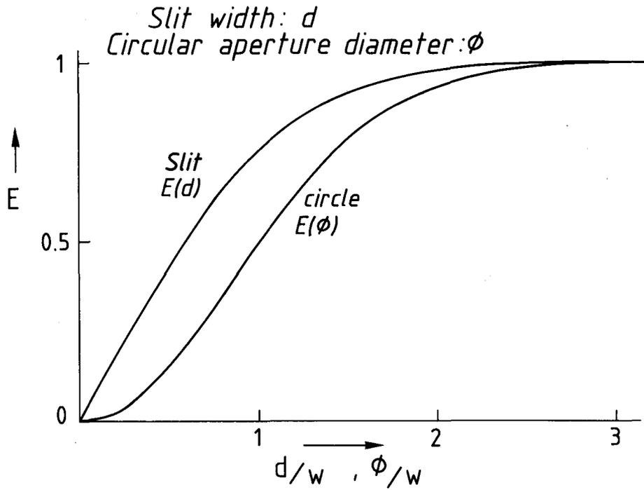
Fig. 2 Energy passed by an aperture for a Gaussian point spread function of FWHM :  $W$
