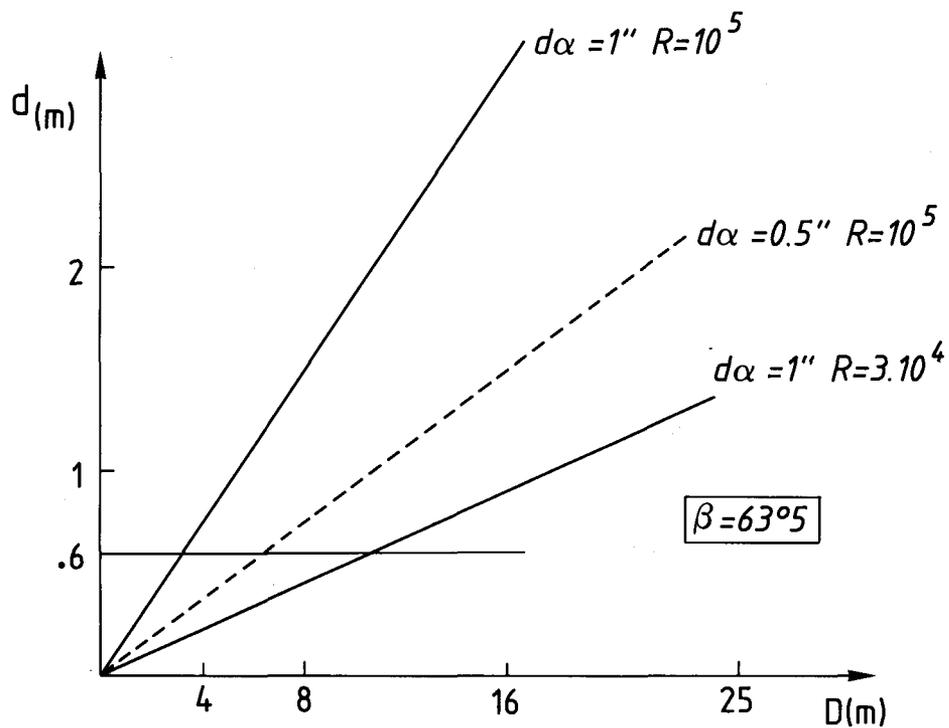
Fig. 8 Grating height versus telescope diameter (slit width is set  $1.5 \times \text{FWHM}$  of seeing disc  $d\alpha$ )
