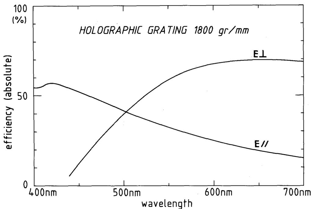
Fig. 9 Measured absolute efficiency of a commercial holo-grating
