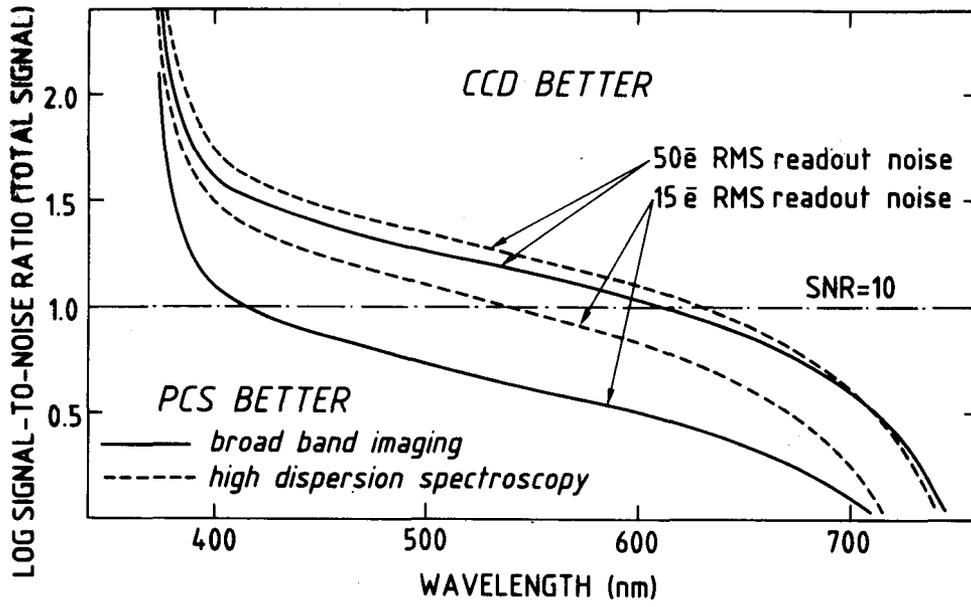
Fig. 1 Signal to noise ratio for equivalent CCD and PCS performance
