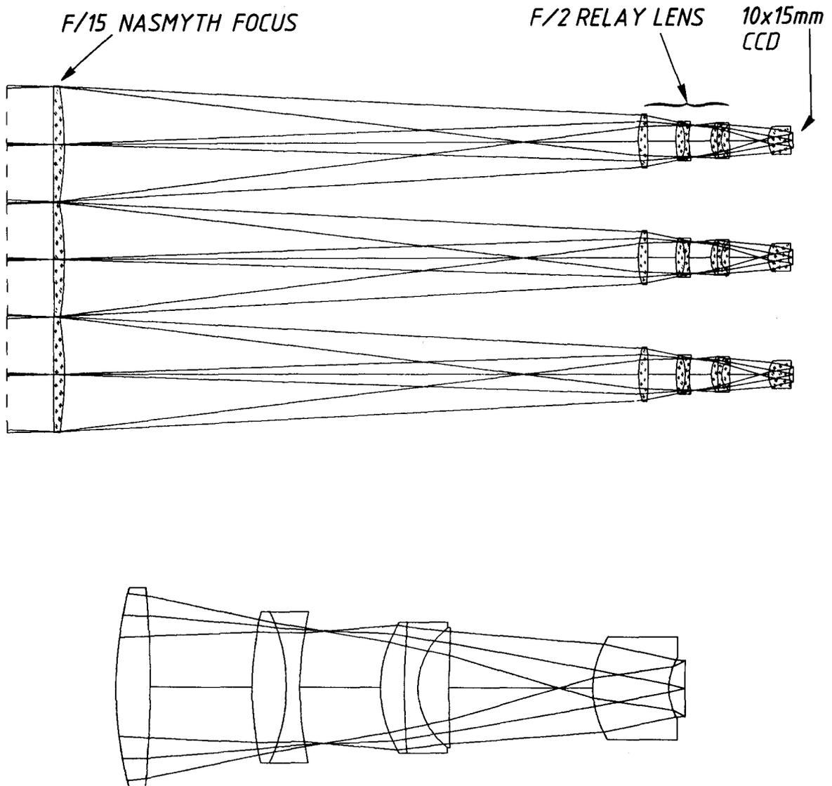
LARGE FIELD IMAGING AT NASMYTH FOCUS USING THE FIELD SLICING TECHNIQUE (F/2)
