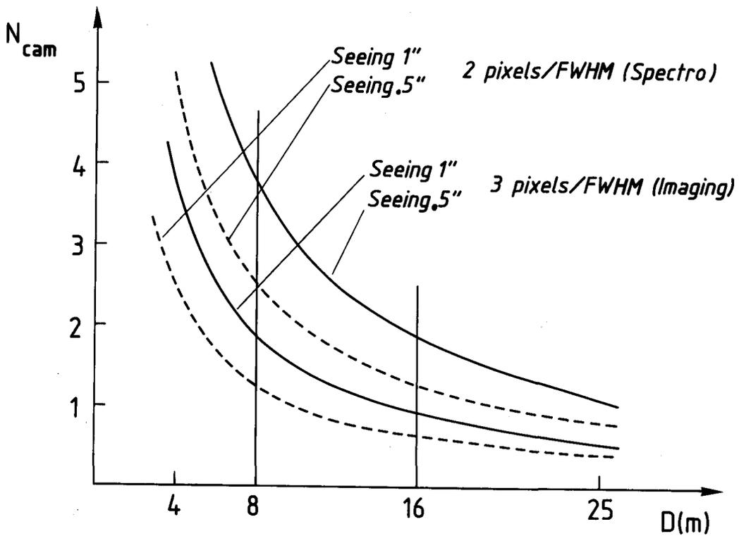
Fig. 4 Camera/Telescope relative aperture for various seeing conditions and a match of 2 and 3 pixels/image element
