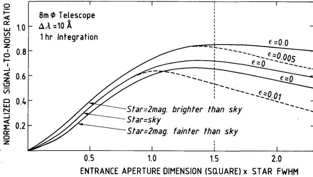
Fig. 3 Signal to noise ratio and spectrograph aperture
