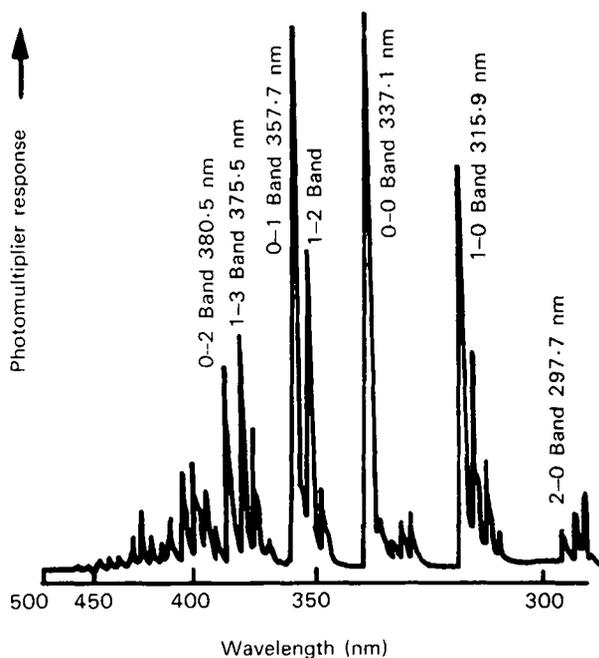
Fig. 1. Emission spectrum of natural nitrogen (0.37 atoms %  $^{15}\text{N}$ ).
