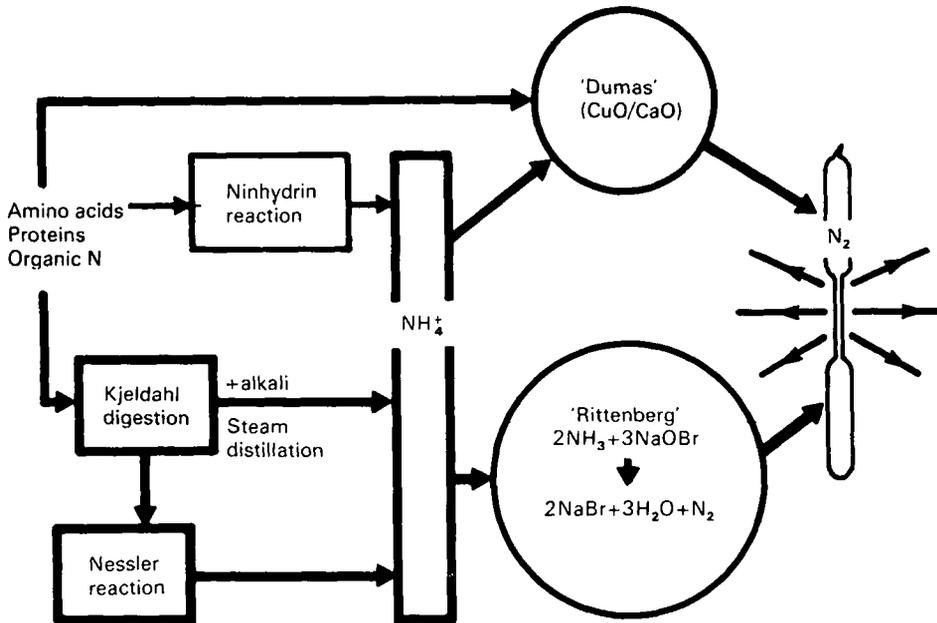
Fig. 3. Preparation of emission tube containing  $\text{N}_2$  for  $^{15}\text{N}$  analysis.
