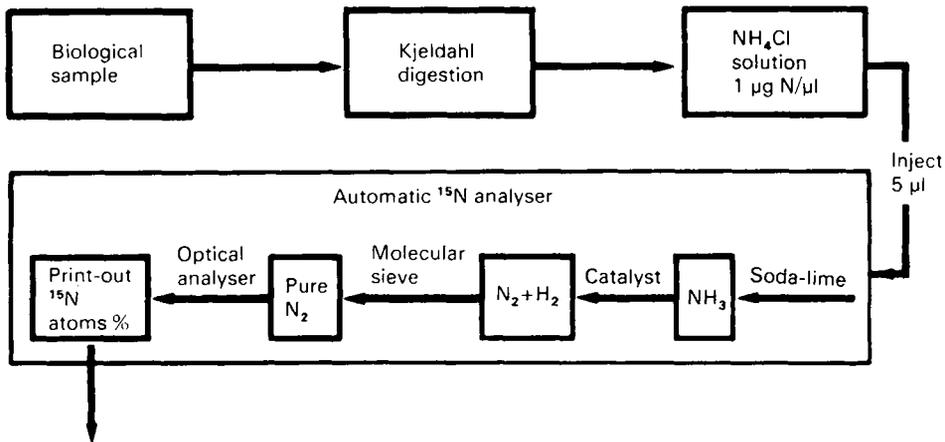
Fig. 4. Method of processing samples and measurement of  $^{15}\text{N}$  in the NIRD automatic  $^{15}\text{N}$  analyser.
