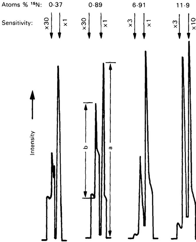
Fig. 2. Emission spectrum of natural and  $^{15}\text{N}$ -enriched nitrogen (2-o transition).
