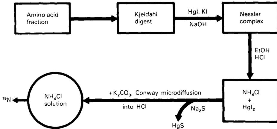
Fig. 5. Method of preparing small quantities of  $N_2$  from amino acid fractions for optical  $^{15}N$  analysis (adapted from Lloyd-Jones *et al.* 1977).
