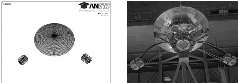
**Figure 1.** Test case and real Pioneer 10/11 geometry (picture courtesy Craig Markwardt).
