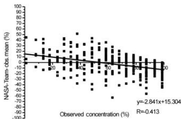
**Fig. 5.** The observed sea-ice concentration vs the ice concentration derived from NASA-Team algorithm minus the mean of the observed data. This plot represents data from all four of the regions in Figure 4 combined. The solid line represents a linear fit of the data, and the dashed lines represent 95% confidence levels.
