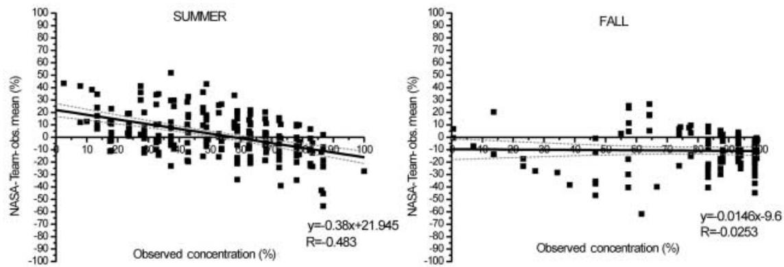
**Fig. 6.** Trends by season of the observed sea-ice concentration vs the ice concentration derived from NASA-Team algorithm minus the mean of the observed data. The solid line represents a linear fit of the data, and the dashed lines represent 95% confidence levels.
