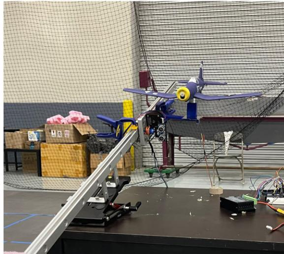
Figure 2. Linear rail system with hinged F4U-Corsair.
