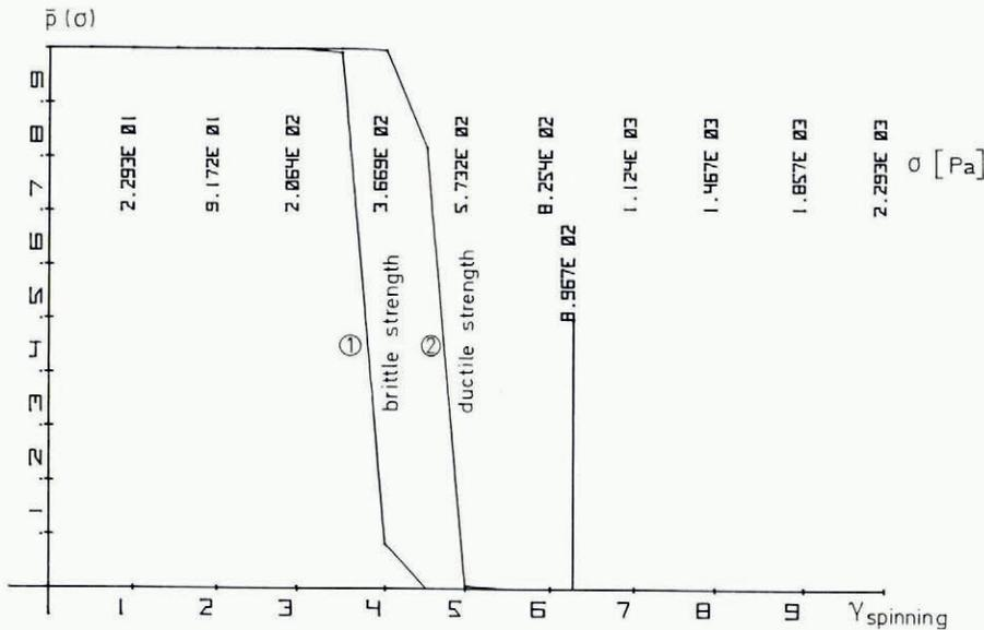
Fig. 8. Simulation of centrifugal tensile strength as a function of link density for two types of similar ductile strength and density. 1:  $n = 10^{11} m^{-3}$ ,  $s_m = 6 \times 10^{-5} N$ ; 2:  $n = 10^8 m^{-3}$ ,  $s_m = 6 \times 10^{-3} N$ .
