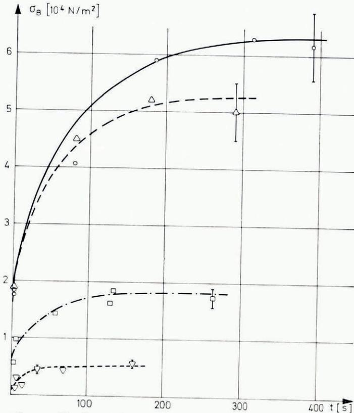
Fig. 10. Tensile strength measured by the centrifugal method as a function of the time between the start of the centrifuge and failure of the sample for different types of snow.
