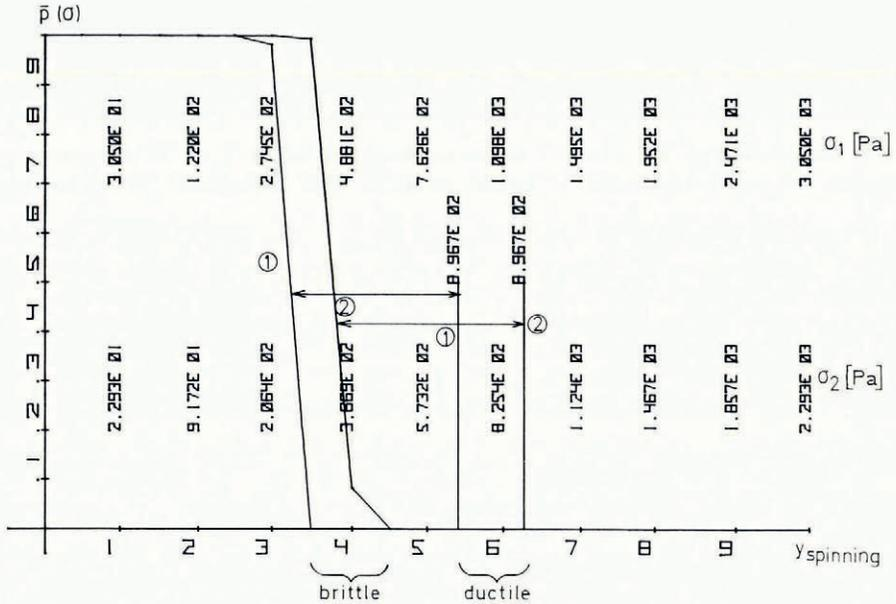
Fig. 9. Simulation of centrifugal tensile strength tests as a function of sample size. The ratio of the cross-sectional areas of sample 1 to sample 2 amounts to 4. The corresponding ratios of ductile to brittle strength are: for the larger sample 2.9, for the smaller sample 2.6.
