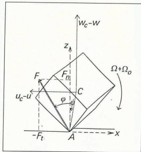
Fig. 1. A grooving stone is modelled as a cube. Notations as used in the text. In this case  $\psi$  and  $d\psi/dt$  are positive.
