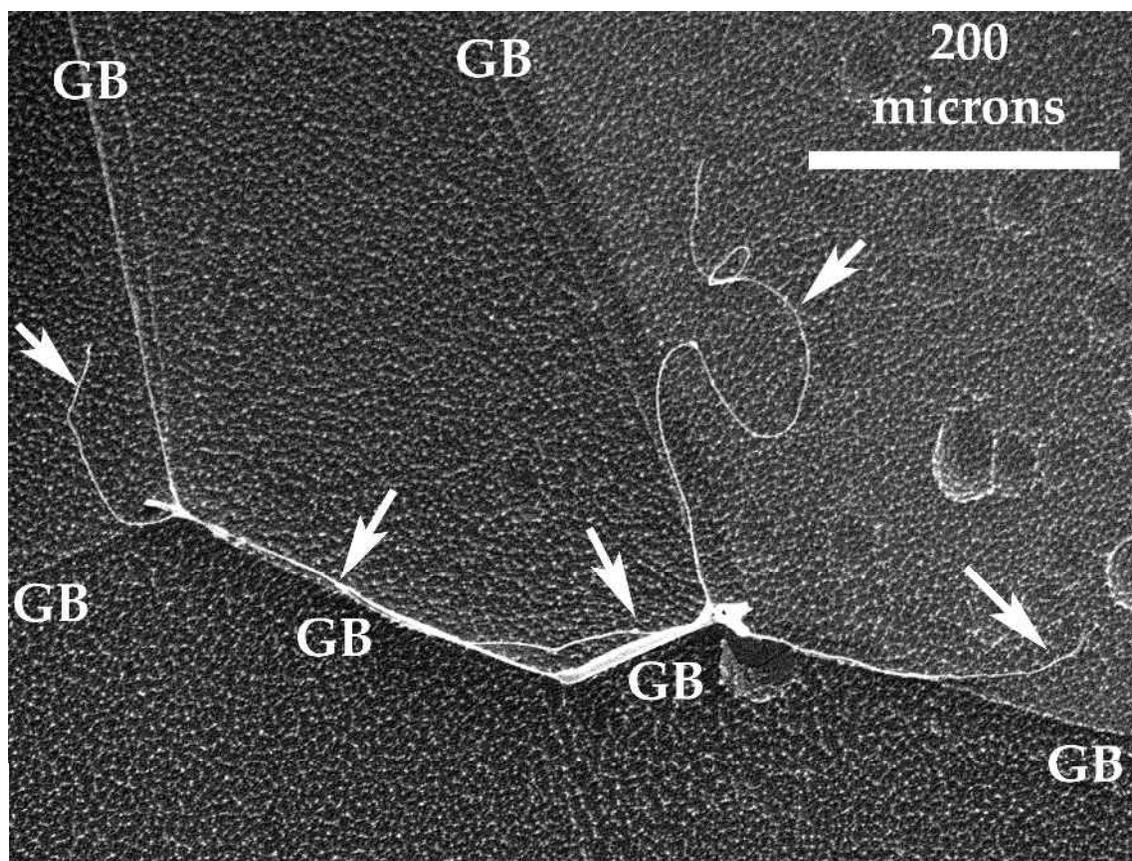
Fig. 1. SE image showing NaCl filaments (arrowed) which arose from the grain boundaries (GB) in 214 m GISP2 ice after 1 hour at 253 K. Note that some of the filaments are no longer fully attached to the grain boundaries since they move due to heating from the electron beam. From Cullen and Baker (2000).
