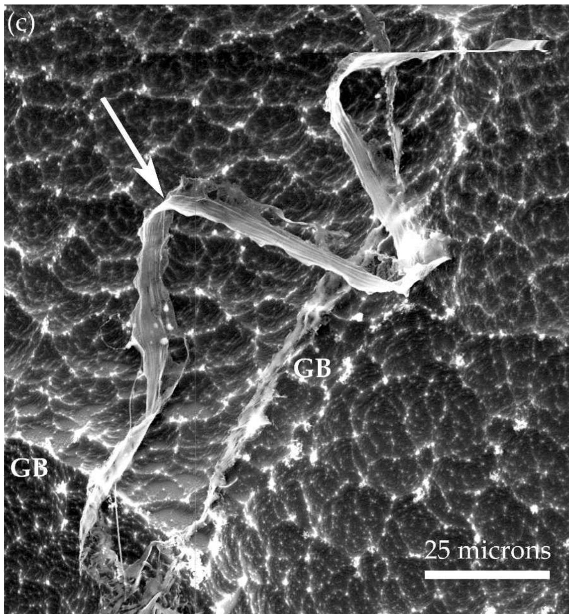
Fig. 3. (a) SE image after sublimation for 20 min at 183 K in the SEM (ice sublimated is approximately 0.1 mm); (b) typical X-ray spectrum from the grain boundary; (c) SE image of ribbon-like NaCl filament (arrowed) from grain boundary (GB) indicated in (a) after sublimation for ~40 min at 183 K (ice sublimated is approximately 0.15 mm).
