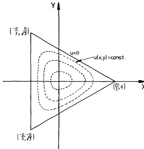
FIGURE 3. *Equilateral triangular plate idealized by four elements*
