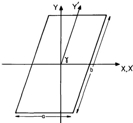
FIGURE 5. Skew-shaped plate
