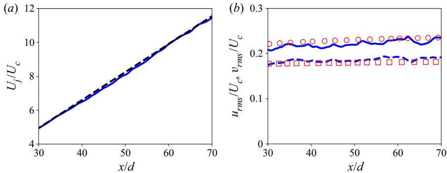
Figure 1. Self-preservation in mean and fluctuations of velocity in a single round jet at  $Re = 11\,000$  compared with the experiment of Panchapakesan & Lumley (1993). (a) Reciprocal of centreline velocity: LES (—, blue); experiment (---, black). (b) Velocity fluctuations: LES,  $u_{rms}$  (—, blue); LES,  $v_{rms}$  (---, blue); experiment,  $u_{rms}$  (○, red); experiment,  $v_{rms}$  (□, red).
