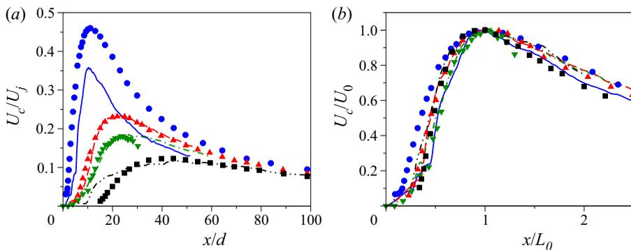
Figure 11. Development of streamwise velocity along configuration axis  $y = 0, z = 0$  for  $2 \leq S/d \leq 8$ . (a) Scaled with input parameters;  $U_c(x)$ . (b) Scaled with peak velocity  $U_0$  and distance to peak  $L_0$ ;  $U_c(x)$  scaled with  $U_0$  and  $L_0$ . For LES:  $S/d = 2$  (—, blue), 4 (---, red), 5 (-•-, green), 8 (-••-,). For experiment (Harima *et al.* 2001):  $S/d = 2$  (•, blue), 4 (▲, red), 8 (■). For experiment (Okamoto *et al.* 1985):  $S/d = 5$  (▼, green).
