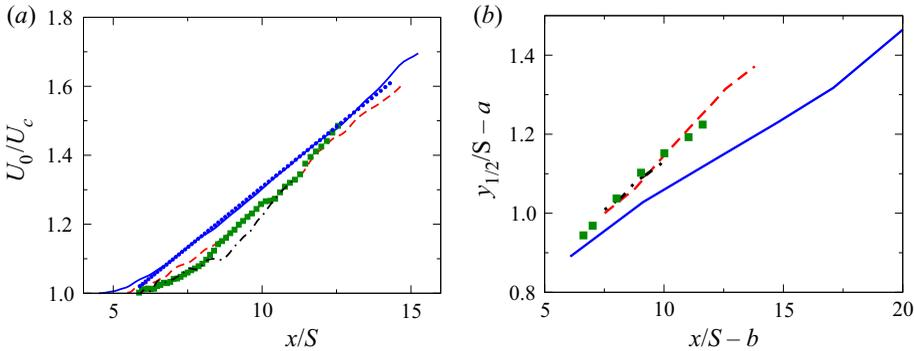
Figure 15. Development of (a) mean centreline velocity and (b) half-width. Here,  $S/d = 2$  (—, blue), 4 (---, red), 5 (■, green), 8 (●—●—, black). Linear fit to the velocity development for  $S/d = 2$  in panel (a) above is shown as a dotted line. Curves in panel (b) have been translated to show the nearly similar development for  $S/d = 4, 5, 8$ .
