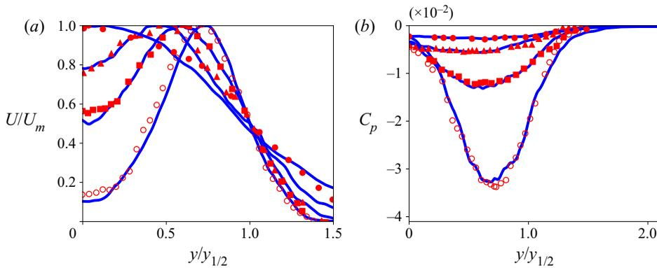
Figure 8. Radial profiles of mean streamwise velocity and pressure coefficient for case TR255: blue curves, LES; symbols (experiment, Okamoto *et al.* 1985) at  $x/d = 10$  ( $\circ$ , red), 20 ( $\blacksquare$ , red), 28 ( $\blacktriangle$ , red), 48 ( $\bullet$ , red). (a) Streamwise velocity. (b) Pressure coefficient.
