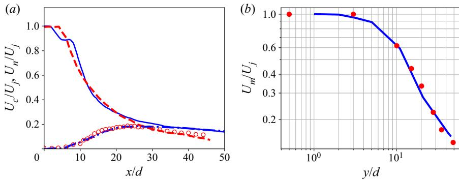
Figure 6. Development of mean streamwise velocity for case TR255. (a) Decay compared with measurement along nozzle axis:  $U_n$ , LES (—, blue);  $U_n$ , experiment (---, red);  $U_c$ , LES (●, blue);  $U_c$ , experiment (○, red). (b) Maximum at any cross-section, initially within individual jets and along  $x$ -axis after jets merge:  $U_n$ , LES (—, blue);  $U_c$ , experiment (●, red).
