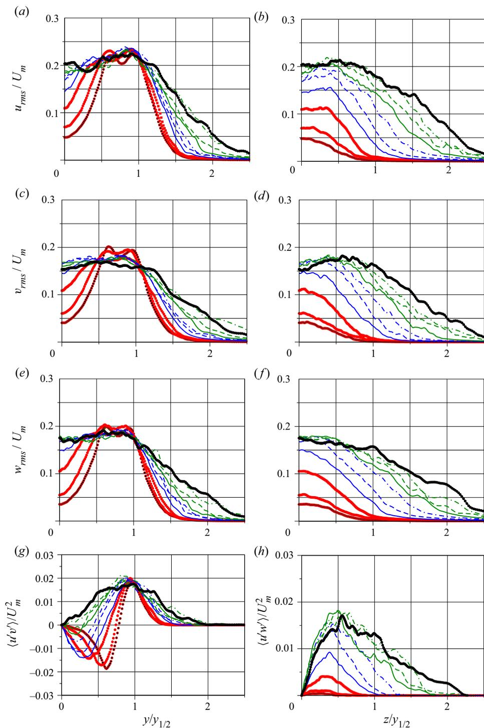
Figure 9. (a–f) Fluctuation profiles and (g,h) Reynolds shear stress profiles. All are normalized with maximum of local mean streamwise velocity  $U_m$  and distance  $y_{1/2}$ . Here,  $x/d = 8$  (○, red), 10 (●, red), 15 (■, red), 20 (—, blue), 25 (---, blue), 30 (-●-, blue), 35 (—, green), 40 (---, green), 45 (-●-, green), 50 (-○-).
