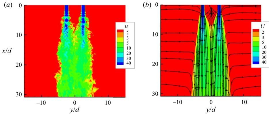
Figure 5. Streamwise component of velocity on plane  $z = 0$  from LES of case TR255. (a) Streamwise velocity  $u(x, y, 0, t)$  ( $\text{m s}^{-1}$ ). (b) Mean streamwise velocity  $U(x, y, 0)$  ( $\text{m s}^{-1}$ ) and streamlines.
