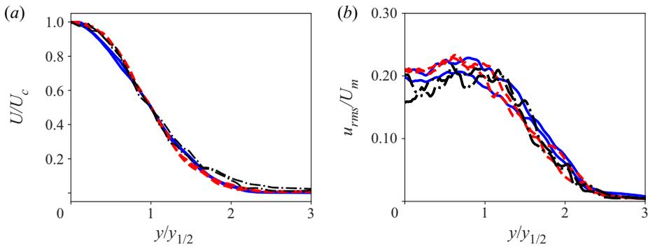
Figure 14. Spanwise profiles of (a) mean streamwise velocity ( $U/U_c$ ) and (b) fluctuations ( $u_{rms}/U_m$ ). Here,  $S/d = 2, x/d = 30, 40$  (—, blue);  $S/d = 4, x/d = 45, 50$  (---, red);  $S/d = 8, x/d = 70, 80$  (-●-●-).
