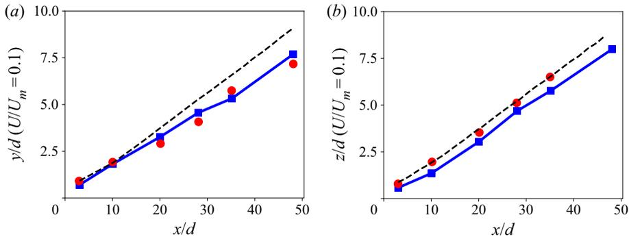
Figure 7. Jet spreading in two planes. Jet boundary is located where mean velocity  $U$  is 10% of the maximum over cross-section ( $x$ , constant): experiment ( $\bullet$ , red); LES ( $\blacksquare$ , blue); single jet ( $---$ ). (a) On  $z = 0$  and (b) on  $y = S/2$ .
