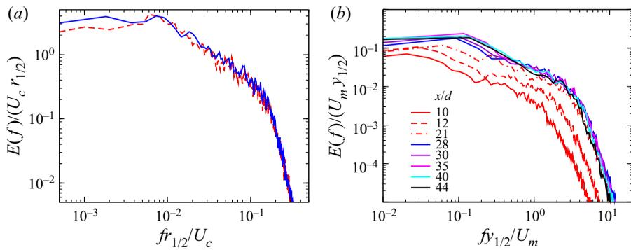
Figure 3. Power spectral density  $E(f)$  of streamwise velocity component  $u(x, 0, 0, t)$ . Scaled with local scales  $U_c$  and  $r_{1/2}$  (case SR120), and  $U_m$  and  $y_{1/2}$  (case TR255). (a) Single jet,  $x/d = 35$  (---, red),  $48$  (—, blue). (b) Twin jet.
