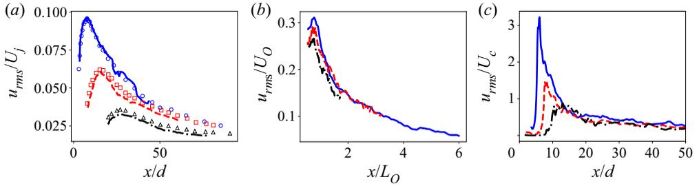
Figure 13. Development of streamwise velocity fluctuations along configuration axis  $y = 0, z = 0$  from LES (a) scaled with  $U_j$  and  $d$ , (b) scaled with  $U_0$  and  $L_0$ , (c) scaled with  $U_c$ . Here,  $S/d = 2$  (—, blue), 4 (---, red), 8 (-●-●-). Data from experiments (Harima *et al.* 2005) in (a) with  $S/d = 2$  (○, blue), 4 (●, red), 8 (■).
