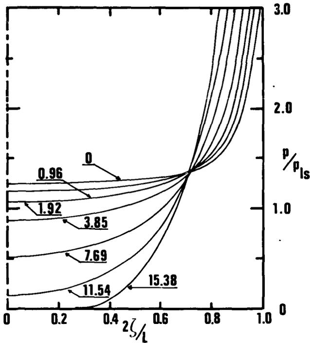
Figure 5.  $p/p_{1s}$ , hydrostatic pressure effect on finite length solid cylinder shrunk-fit into elastic region, for  $\nu_c = \nu_r = 0.3$ ,  $G_r = G_c$ ,  $L = 1.0$  and various  $h$ .
