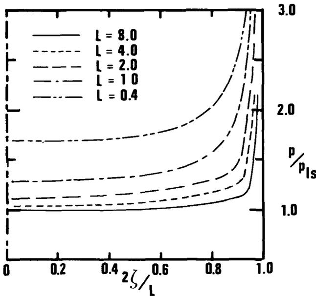
Figure 2.  $p/p_{1s}$ , finite length solid cylinder shrunk-fit into elastic region, for  $\nu_c = 0.5$ ,  $\nu = 0.3$ ,  $G_c = G$ , and various  $L$ .
