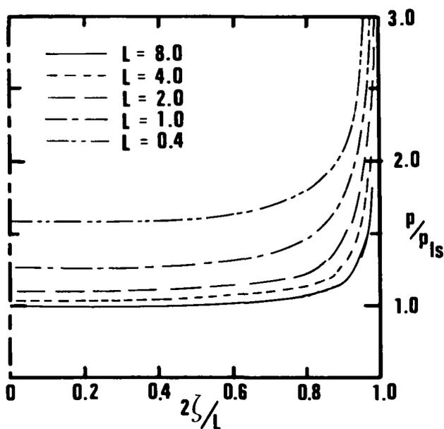
Figure 1.  $p/p_{ls}$ , finite length solid cylinder shrunk-fit into elastic region, for  $\nu_c = \nu_r = 0.3$ ,  $G_c = G_r$ , and various  $L$ .
