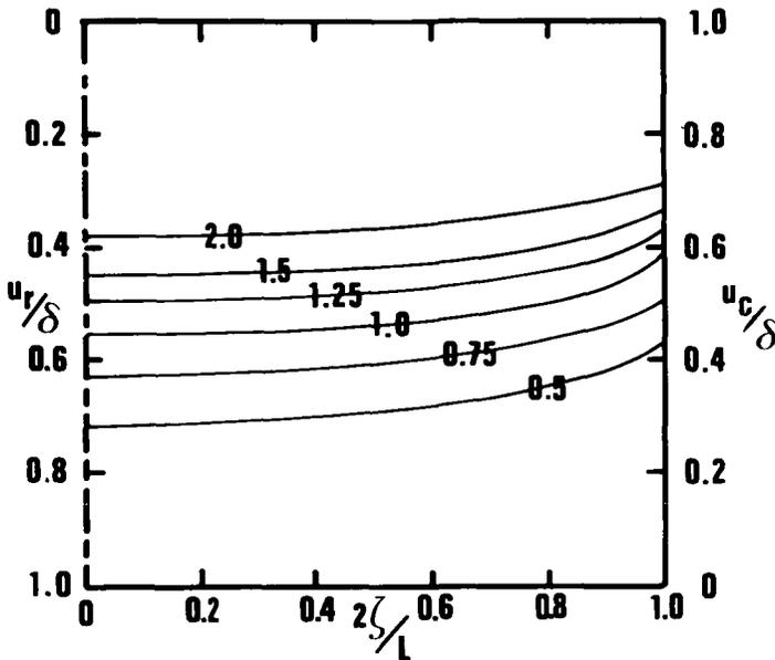
Figure 3.  $u_c/\delta$  and  $u_r/\delta$ , finite length solid cylinder shrunk-fit into elastic region, for  $\nu_c = \nu_s = 0.3$ ,  $L = 1.0$  and various modular ratio  $G_c/G_s$ .
