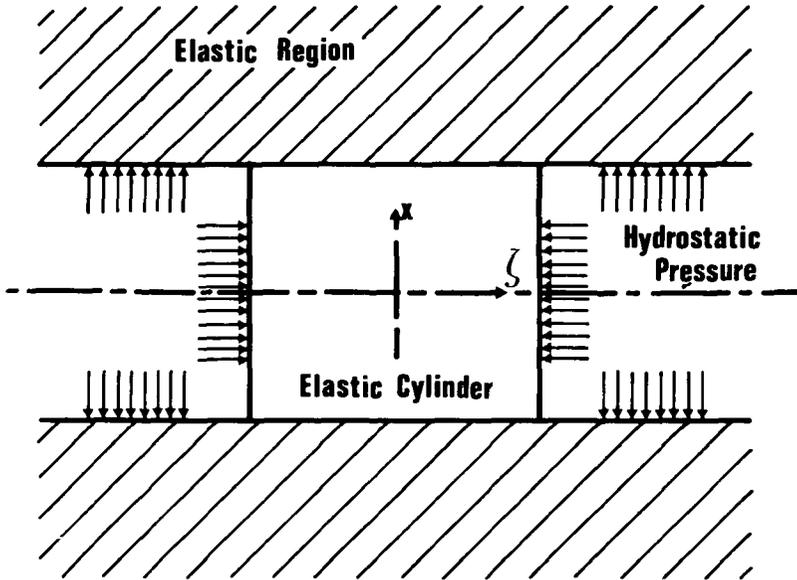
Figure 4. Finite length solid cylinder shrunk-fit into infinite elastic region with hydrostatic pressure acting.
