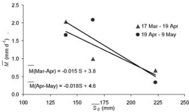
Fig. 6. Association between landscape-class melt rate and average pre-melt SWE in complex tundra landscapes, Granger sub-catchment (<5 km<sup>2</sup>), 1999. The two linear relationships between pre-melt SWE and melt rate shown are similar enough that coefficients and constants could be averaged.
