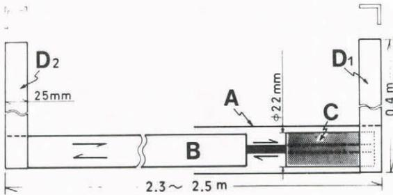
Fig.3. Long-span deformation gauge.
