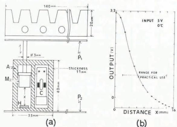
Fig.2. Short-span deformation gauge. a: the gauge; b: characteristics.
