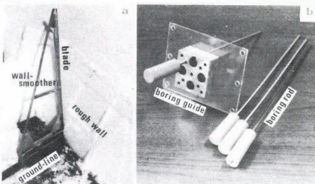
Fig.1. Instruments for Hole-mark method. a: wall-smoother, b: 5-hole boring device.
