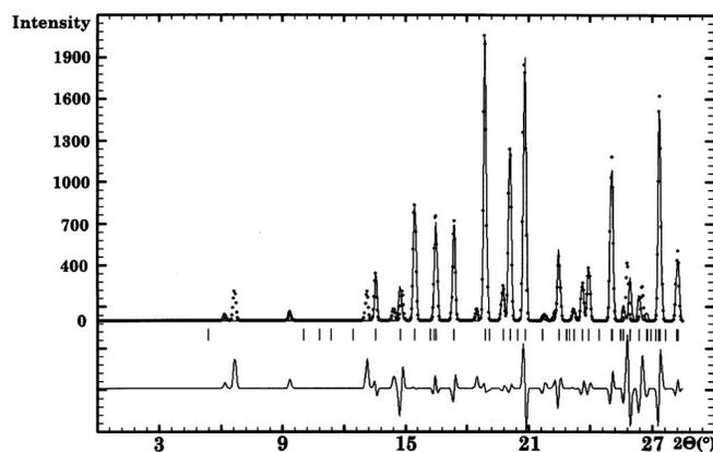
Figure 5. Idealized powder pattern with Gaussian peak shape, reconstructed from PDF 43-1748, bethanechol chloride, at the end of the McMaille execution (after correction of a  $-0.10(2\theta)^\circ$  zeropoint), displayed by WinPLOTR. There are 8 unexplained lines among the first 26 observed ones. The first four lines at low diffraction angle are half of these impurity lines. This does not preclude McMaille to find the correct cell in first position.
