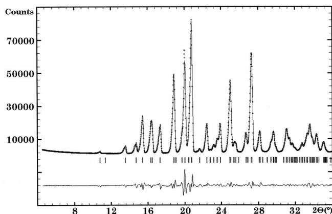
Figure 4. Le Bail fit on the powder pattern of bethanechol chloride (using FULLPROF,  $P2_1/n$  space group). Sample dusted through a sieve on a silicon zero-background holder with a slight pressure by a sheet of paper in order to obtain a better plane surface. Preferred orientation is not completely removed, these conditions lead to a lower resolution with FWHM  $\sim 0.25(2\theta)^\circ$ .
